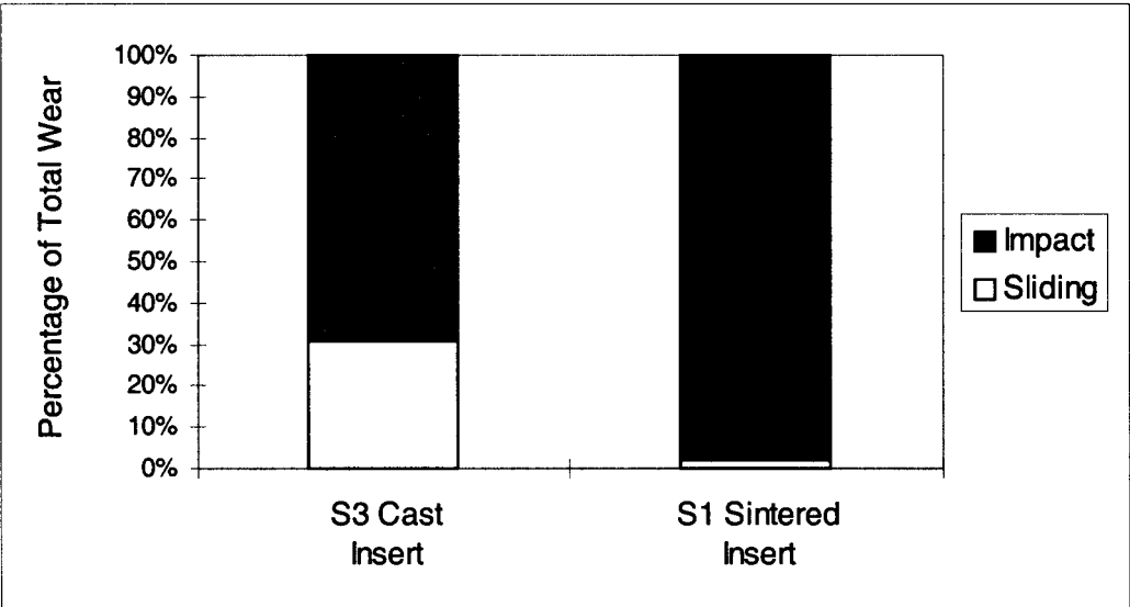
Fig. 7.13 Percentage of total wear caused by impact and sliding for a cast seat insert (S3) engine test
