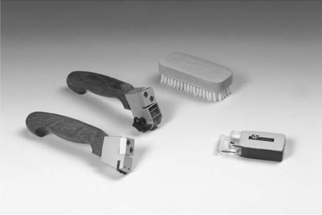
Fig. 12.65 Hand cutting tools (source: Byk-Gardner).
