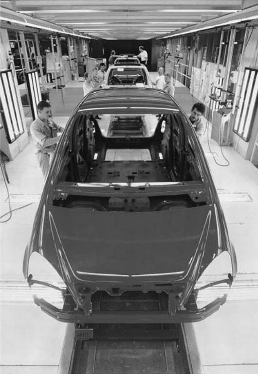
**Fig. 11.1** Inspection zone of an automotive coating line (source: BASF).
