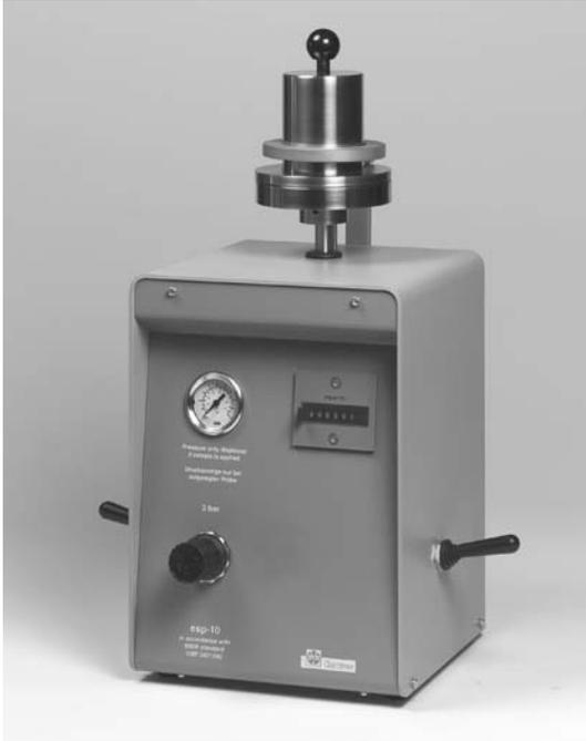
Fig. 12.75 Single-impact tester (source: Byk-Gardner).
