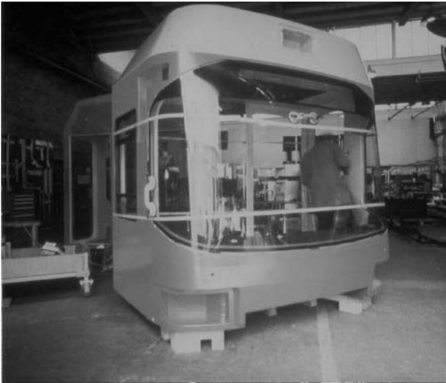
Fig. 10.31 Glazing of front cabin of a tram.
