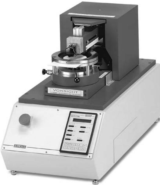
Fig. 12.66 Automatic cross-cut equipment (source: Erichsen).
