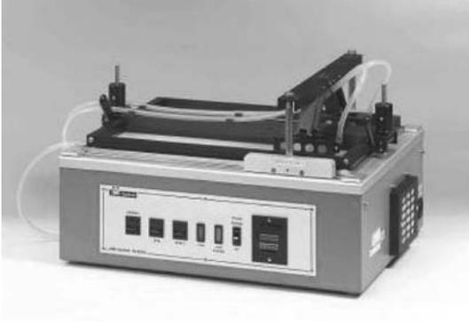
**Fig. 12.81** Abrasion scrub tester (source: Byk–Gardner).
