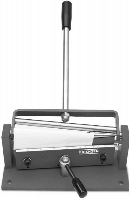
**Fig. 12.71** Conical mandrel (source: Erichsen).
