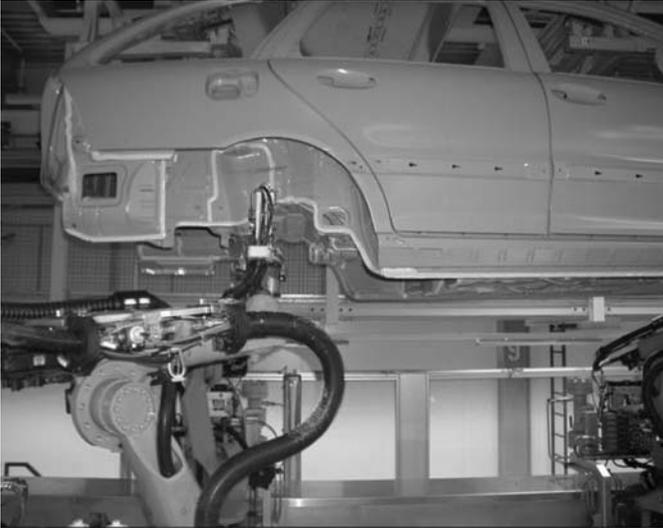
**Fig. 8.3** Application of under body protection material.
