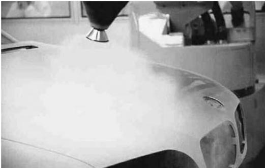
Fig. 6.22 Bell application of powder clear coat. (source: BMW)
