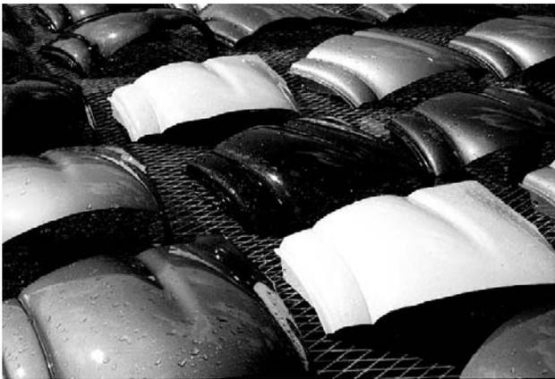
Fig. 12.39 Example of specimen for weatherability tests.
