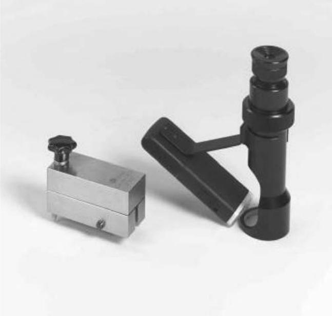
**Fig. 12.60** Buchholz test equipment (source: Byk–Gardner).
