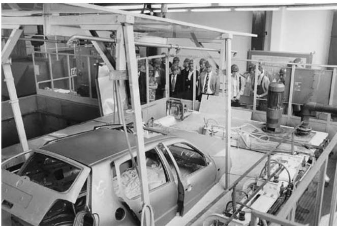
Fig. 12.54 Pilot electrocoat tank (source: BASF).
