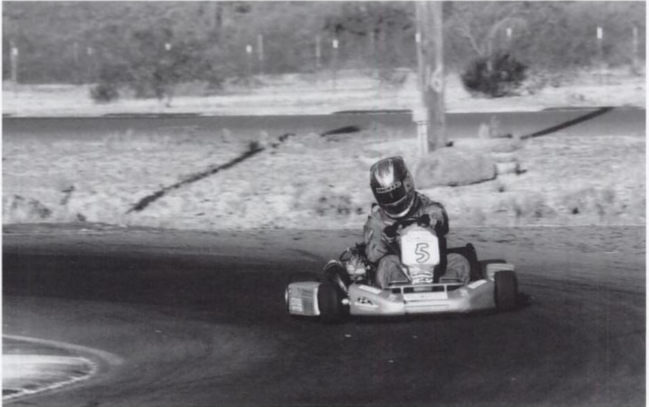
When a kart is understeering, the front tires are sliding more than the rear tires, and the kart tends to plough straight ahead.
