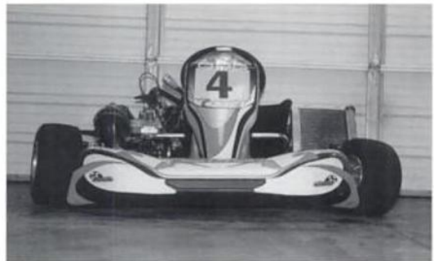
This photo shows the effect of castor. When the front tires are turned to the left, the left-side tire is driven downward, lifting that corner of the chassis, while the right front tire rises, lowering that side of the chassis. This unloading of the chassis on the inside of a corner is what takes weight off of the inside rear tire and allows the kart to turn.
