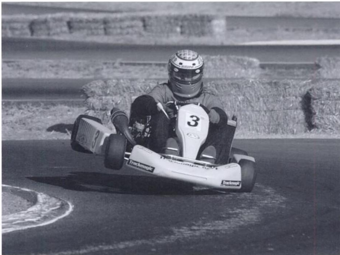
Kart dynamics to the extreme—in this case, a kart “bicycling” around a corner. GO Racing Magazine
