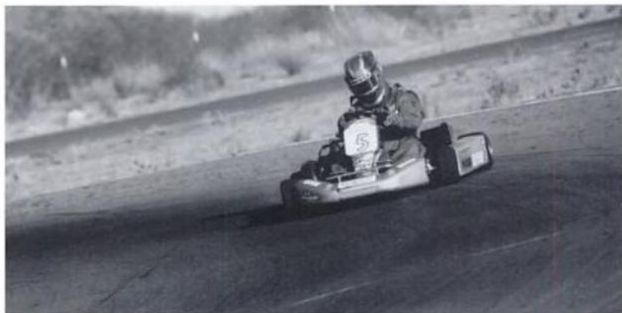
The driver in this photo has entered a corner while trail braking heavily, which has caused the kart to oversteer dramatically. In this case, he has asked the rear tires for more than 100 percent, and they began to slide sideways in response.
