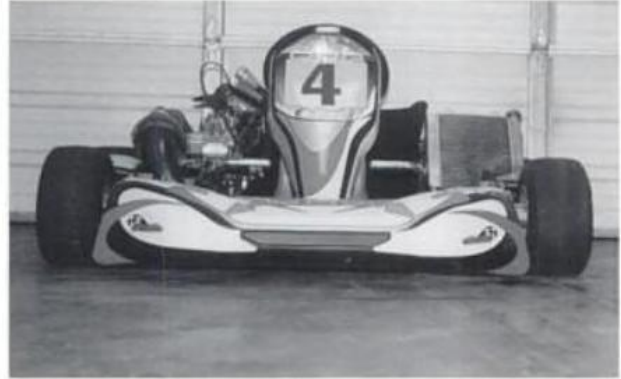
Here the front tires/wheels are pointing straight ahead, and the chassis is level with the ground.
