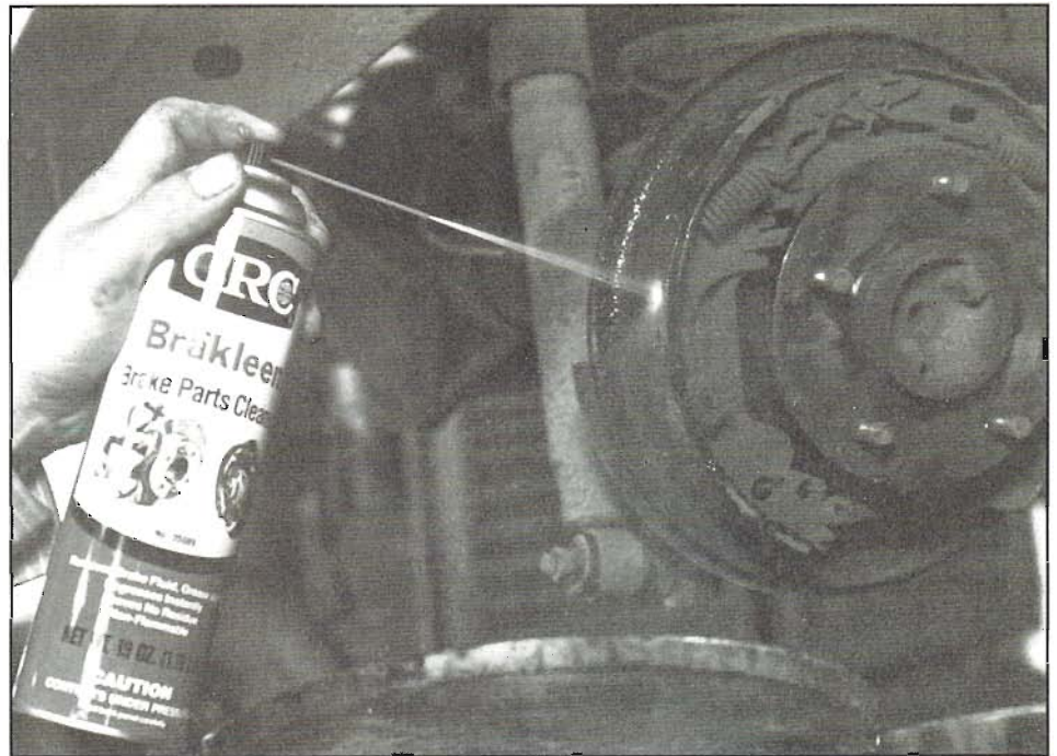
Cleaning brake parts should be done with special brake-cleaning fluid. CRC Brakleen is used at start of brake-maintenance job. Petroleum products should never be used on brake parts, as brake fluid is easily contaminated. Photo courtesy CRC Chemicals.
