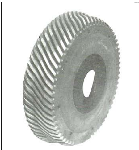
Fins on Alfa-Romeo aluminum/cast-iron drum are designed to pump air between drum and tight-fitting wheel. Drum goes with brake assembly pictured on page 22. Photo by Ron Sessions.
