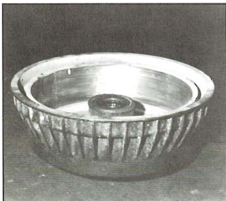
Cast-iron brake drum is large and heavy compared to disc-brake rotor of equal effectiveness. Many '60s and '70s American cars have drums of this type. This front-brake drum has integral wheel hub and bearings.
