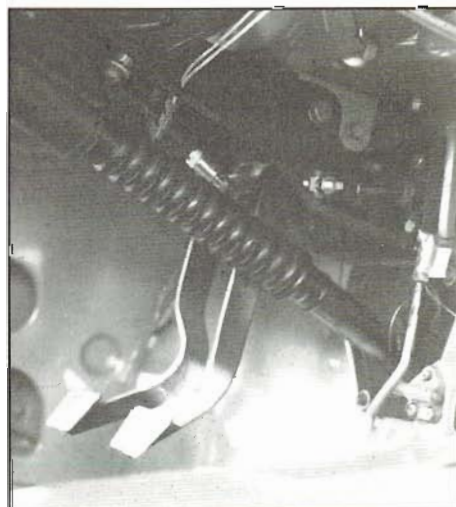
Hanging pedals are neat and package well in most large cars. Such a setup with dual master cylinders can be difficult to adjust, particularly when you're in a hurry—just the place for a remote adjuster.
