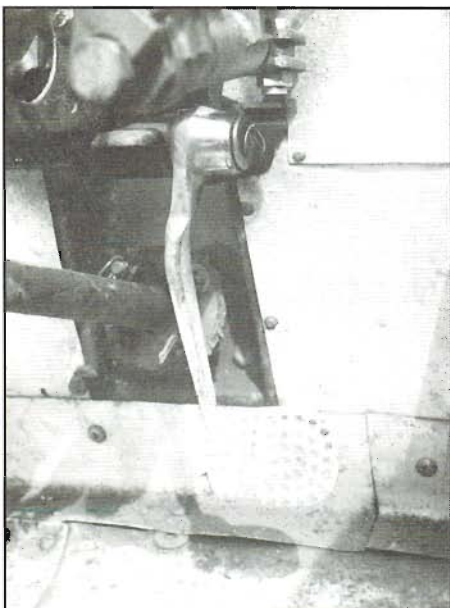
Bad pedal design on homemade race car has pedal arm off-center to pad and pivot housing. When pushed on, twist of arm causes excessive flexibility and higher stresses. If arm were moved to right, pedal would be stiffer and stronger.
