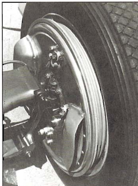
Racers soon discovered that bigger brakes are better. This old Talbot Grand Prix car used 18-in. wheels—brake drums are bigger! Fitting drum into wheel limits its size.
