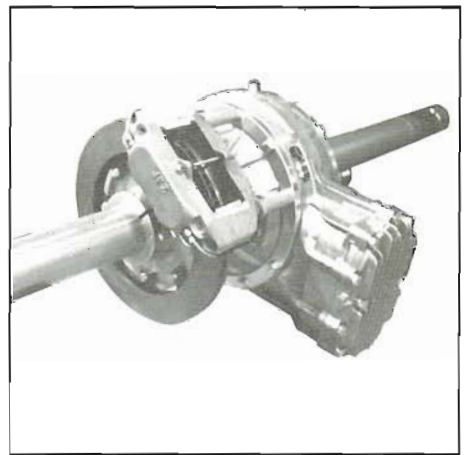
Sprint-car rear axle: Single inboard brake on solid axle is possible because of exposed axle shaft and locked rear end. Not only is weight reduced by one-half, when one wheel hits a bump, brake moves smaller distance than wheel, reducing brake's effective unsprung weight. Improved handling results. Photo by Tom Monroe.
