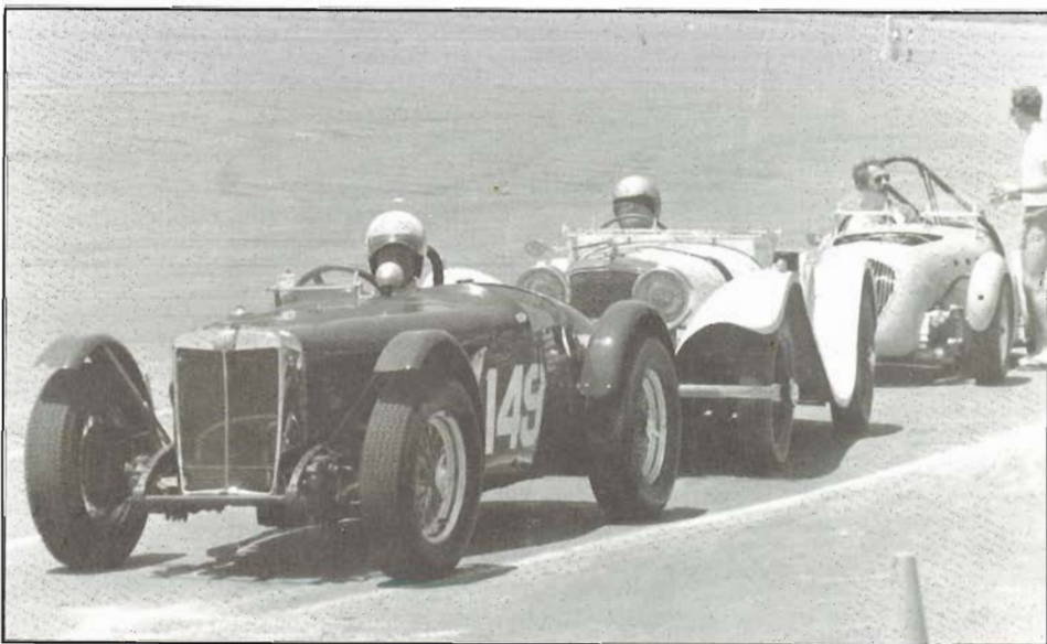
Old sports cars are unstreamlined. Body shapes are rough, angular and have lots of parts sticking into airflow. Streamlining of cars refers to shape, not size of body. An unstreamlined car has a higher drag force on it than a streamlined car of the same size.
