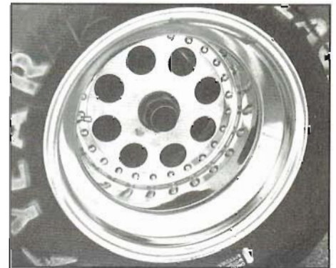
Centerline wheels were originally a solid-center construction. As need to direct cooling air through wheels became evident, these vented versions were created. Because this wheel is so deep, duct should be used to take advantage of cooling holes.
