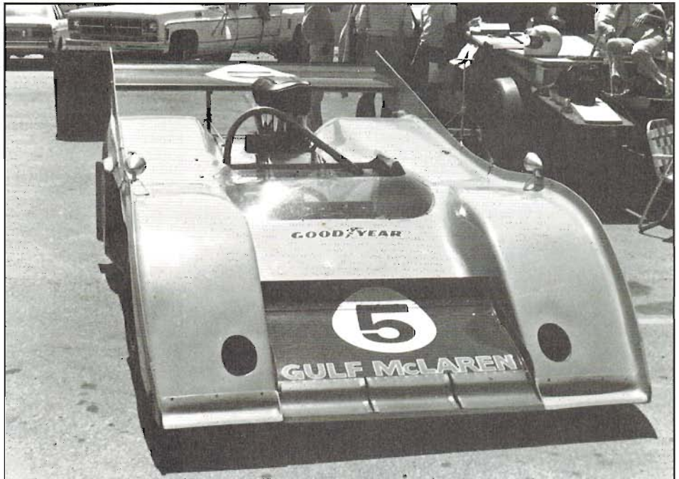
Brake ducts on McLaren Can-Am car are simple holes in body with tubes attached. Forward surfaces of sloping front fenders are in high-pressure areas.
