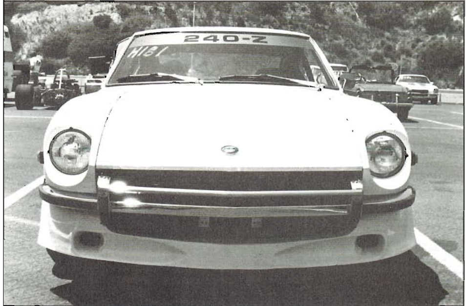
Aftermarket spoiler has holes for brake-cooling ducts. High pressure exists in front of spoiler, making ideal spot for brake ducts. Spoiler without ducts adversely affects brake cooling. On a race car, tubes should be used to route air directly to brakes.
