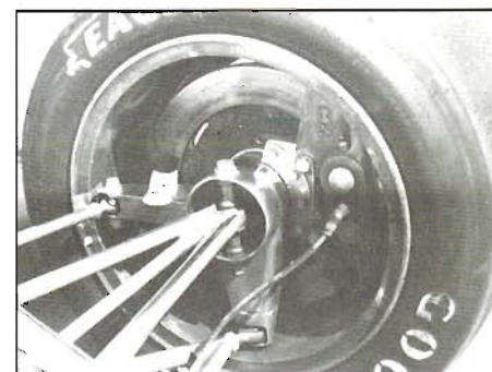
Race cars generally use largest possible brake diameter. On this Indy Car, caliper almost rubs against inside of wheel.
