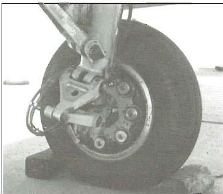
Aircraft multi-disc brake: Brake, which is buried in wheel, is good for one stop after landing. Brake must cool before another landing can be made.
