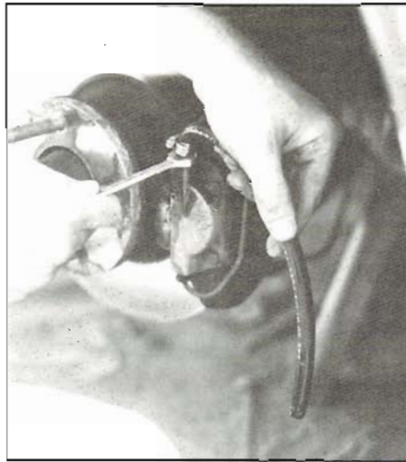
Not a good setup for bleeding brakes: Hose should be clear and free end immersed in fluid in clear bottle or jar. Bubbles can then be seen and mess is avoided.
