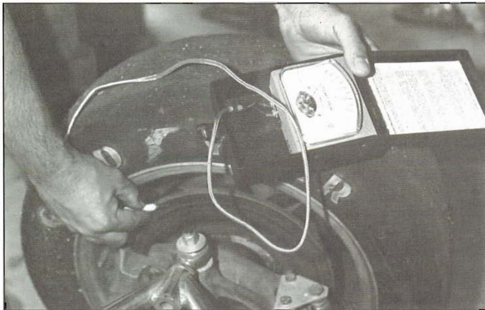
Pyrometer is used to measure brake temperature on open-wheel race car. This is difficult on full-fendered cars. When checking temperature, quickly hold pyrometer probe firmly against rotor until meter needle stops rising. Peak temperature during braking cannot be measured with hand-held pyrometer because some cooling will occur. Peak temperature can only be measured with an onboard pyrometer, or temperature-indicating label or paints.
