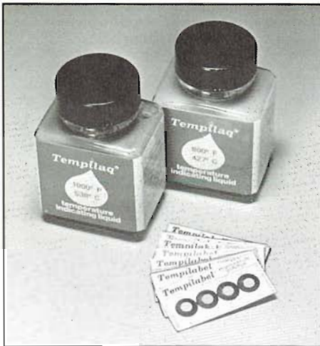
Excellent temperature indicators are manufactured by Tempil. Tempil's Tempilaq paint melts when heated to rated temperature. Tempilabel spots turn black when heated to rated temperature. Photo by Tom Monroe.
