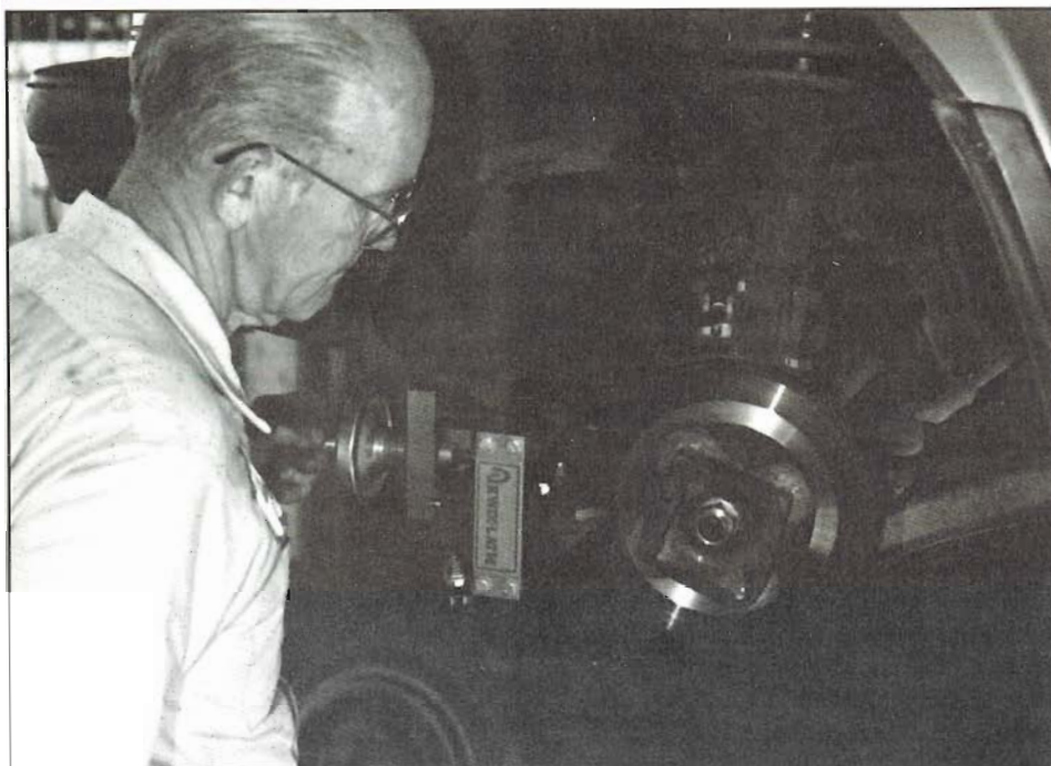
Rotor is being surfaced with tool mounted on car. Rotor can be rotated by engine with this front-wheel-drive car. Tool machines both sides of rotor simultaneously, ensuring that surfaces will be parallel. Rotors that cannot be surfaced on car are removed and done on a special lathe.
