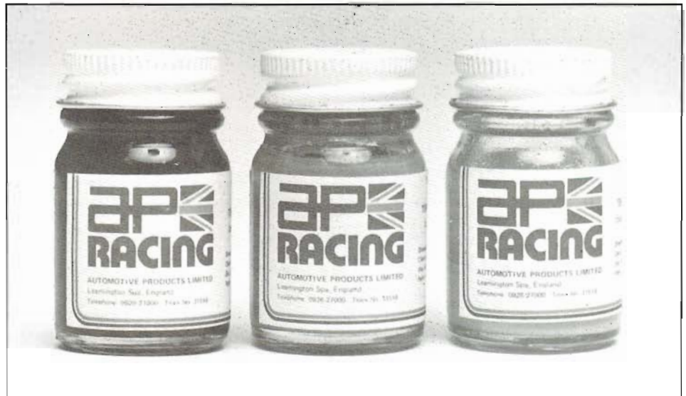
As with other temperature-indicating paints, AP Racing's indicators can be used to check rotor or brake-drum temperature. Temperature indicators will tell you the highest temperature reached, if you use the right range of paints. Courtesy AP Racing.
