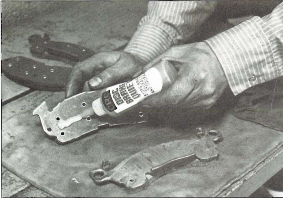
CRC Disc Brake Quiet compound is applied to backside of brake pads to reduce brake noise. CRC recommends using compound on outboard pads. They can be reassembled on the car following a 10-minute curing time. Photo courtesy CRC Chemicals.
