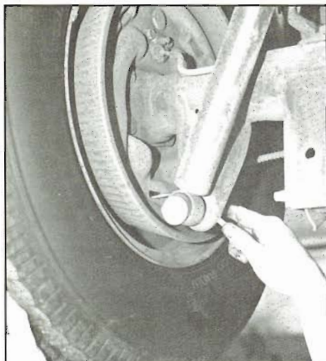
Although duo-servo brake uses automatic adjuster, brakes must be manually adjusted after brake-lining replacement. Blade-type tool is used to turn adjuster through slot in backing plate (arrow).
