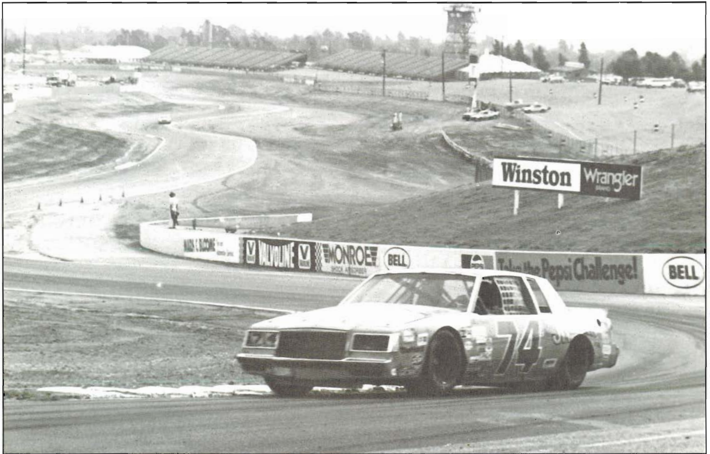
Stock car running on road course is hard on brakes. Stock cars are the heaviest road-racing vehicles, and are powerful. Brake ducts and heavy-duty linings are a must on hot day at Riverside Raceway.
