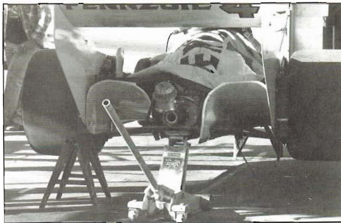
Design of ground-effects car should be left to experts. Wind-tunnel testing is the only sure way to determine aerodynamic loads on car. Note ground-effects exit tunnels at rear of car. Photo by Tom Monroe.
