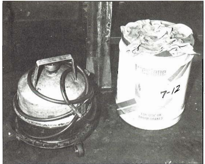
Pressure bleeder is used in most repair shops because of its speed. Huge can of fluid is used to fill pressure bleeder. Because most racers fear possible use of old or contaminated fluid, pressure bleeders are not popular. For road cars, they offer speedy low-cost brake bleeding in a shop.
