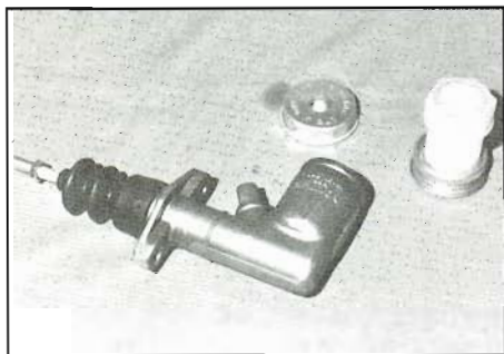
Girling single master cylinder is type found on many race cars, typically in dual master-cylinder setup. It is small, simple and lightweight. White nylon cap/reservoir extension increases reservoir capacity. Cylinders are also used to operate hydraulic clutches.
