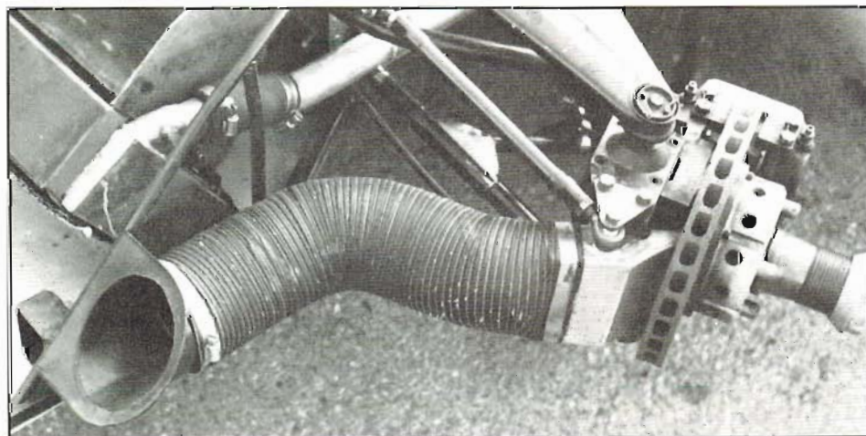
A well designed duct is simple and neat. Ducts sealed to center of rotor such as this are much more efficient than those that just point at center of rotor. Flex hose used for air ducts on cars is available in auto parts or surplus stores. Notice both ends of hose are securely attached with hose clamps.
