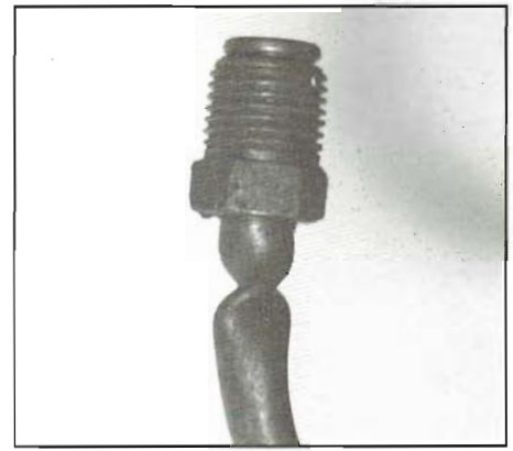
When brake line rusts, fittings can seize on steel tube. This can happen when seized fitting is turned with a wrench. Although such a line may not leak, it should be replaced.
