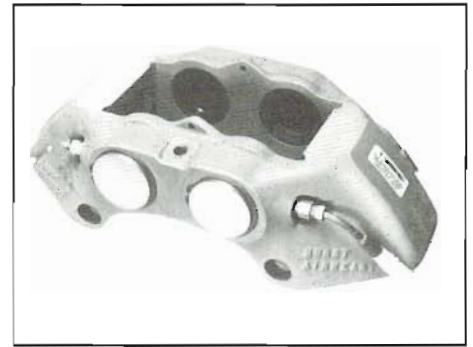
Hurst/Airheart 200X2 caliper is largest one offered by this manufacturer. Brake torque is rated at 23,000 in-lb brake torque at 1200-psi hydraulic pressure. Double-piston caliper is popular for use on racing stock cars. Photo courtesy Hurst Performance.
