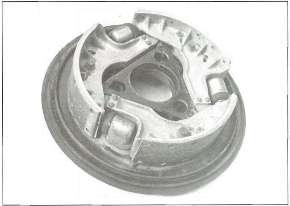
Prior to disc brakes, some drum-brake designs got pretty exotic. This three-leading-shoe drum brake was used on some Alfa Romeo sports cars. Although they did a good job of stopping the little sports cars, they were heavy and complex. Notice that each shoe has its own wheel cylinder.
