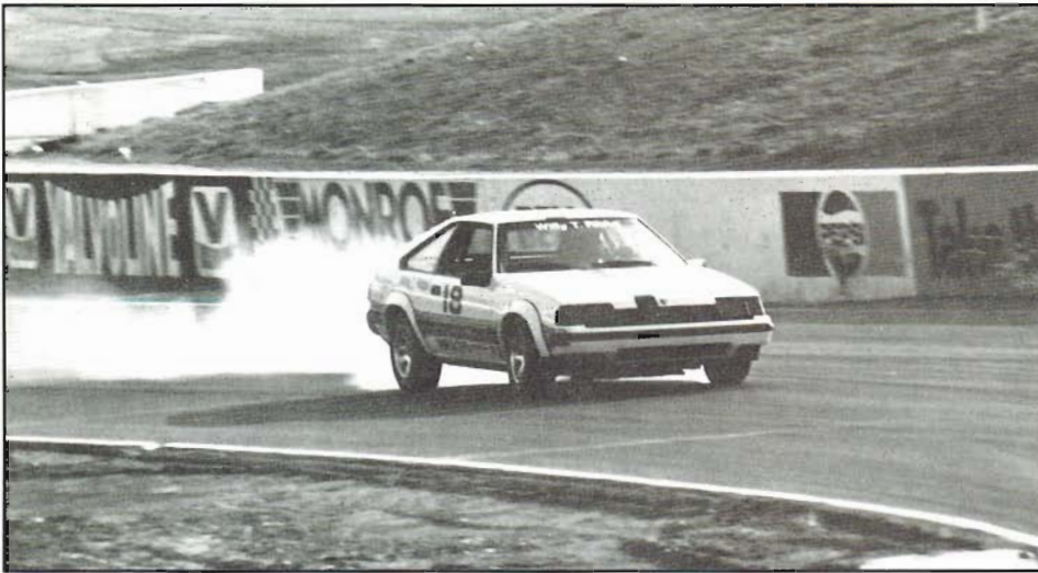
Once wheels are locked, driver's strength is the only thing limiting brake-pedal force. As fear increases, the harder he pushes. This condition represents the maximum force that can be applied to a brake system. Brake-pedal force during a maximum-deceleration, controlled stop is much lower.
