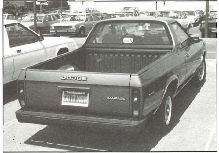
Toughest type of vehicle to maintain brake balance under all loading conditions is nose-heavy, front-wheel-drive pickup. Load-sensing proportioning valve between body and rear axle of Dodge Rampage adjusts brakes so brake balance is maintained under all load conditions.
