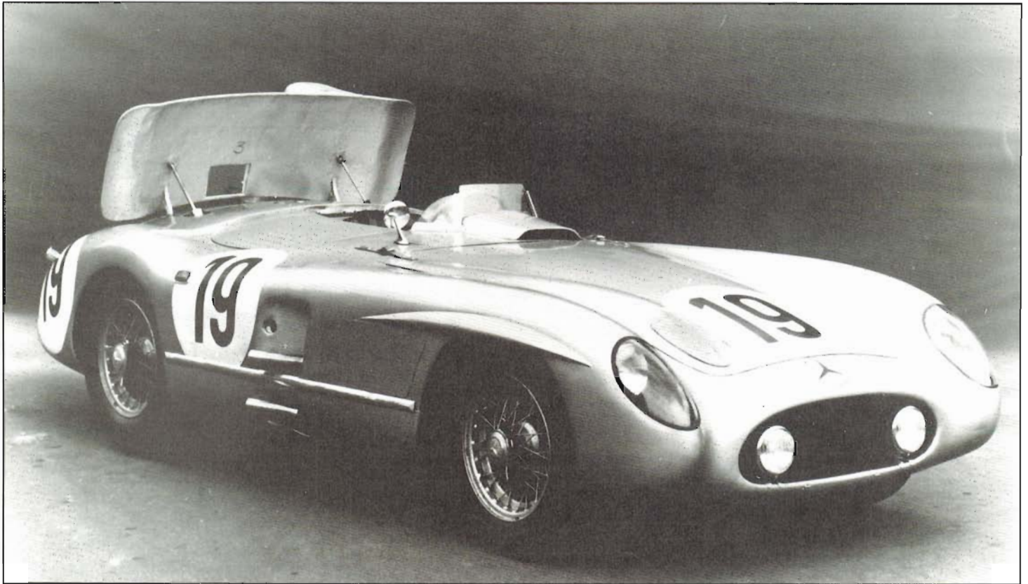
Outlawed by most racing organizations, movable air brakes, such as one at rear of this 1955 300SLR Mercedes, are extremely effective at over 100 mph. Frontal area and drag coefficient are increased dramatically when air brake is activated. Photo courtesy Mercedes-Benz.
