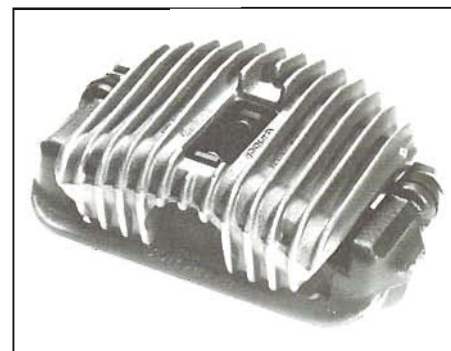
While most road-car brakes are too heavy, some are worth considering for high-performance use. Cast-iron 1984 Corvette sliding caliper was designed more for high performance than low cost. It may be a natural for road car with 4-wheel disc brakes. Photo courtesy Girlock Ltd.
