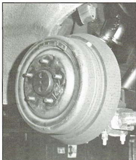
Most production sedans have drum brakes on the rear and disc brakes on the front. Drum brakes are preferred on rear wheels because a parking brake is easily adapted. This large drum is on the rear of a 2-ton sedan.
