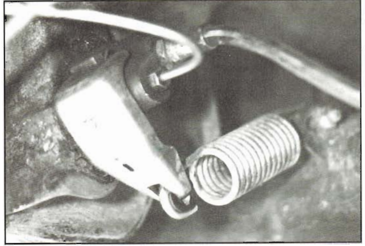
Both proportioning valves are adjusted by spring between rear axle and proportioning-valve lever. Valve adjustment changes with rear-suspension travel from weight on rear wheels. Rear-axle movement moves lever and changes valve setting. As weight on rear wheels increases, so does rear-wheel-brake pressure. Cars that have such large weight-distribution changes, such as this Plymouth Voyager/Dodge Caravan (left) or Peugeot station wagon (right), will benefit from a height-sensing proportioning valve.
