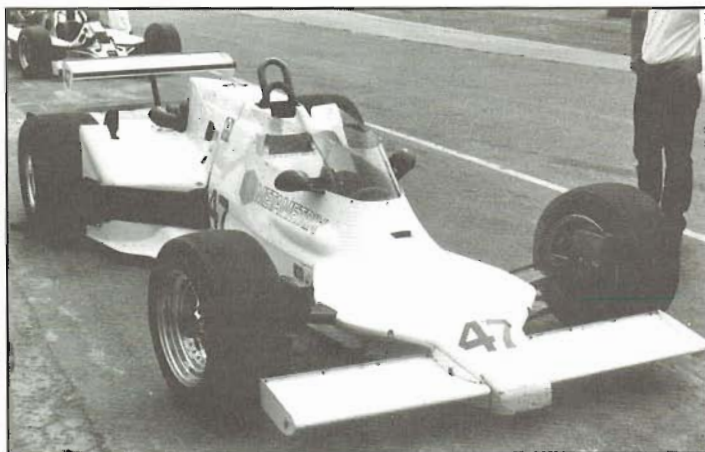
Modern cars with wings and ground effects generate much more downforce than ordinary cars. Indy Car cornering and braking loads are much higher than for a modified road car. You must know speed and downforce to correctly calculate loads generated by tires.
