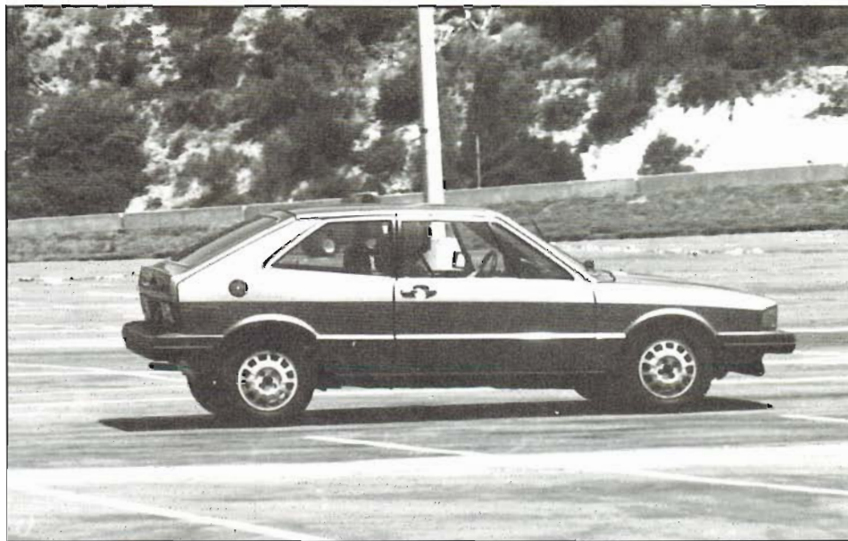
A front-wheel-drive car, such as this VW, has majority of weight at front. When brakes are applied hard, more weight is transferred to the front. The nose drops and tail rises during braking due to weight transfer.
