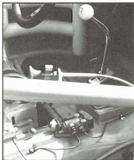
Tilton adjustable proportioning valve is used on this stock car instead of a balance bar. A tandem master cylinder is used for safety. The proportioning valve is mounted on drive-shaft tunnel where driver can easily reach lever. Valve is installed in brake line to rear brakes.
