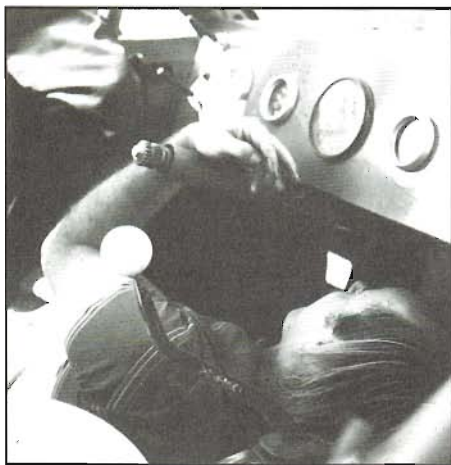
Making under-dash brake-balance adjustment forces mechanic into this uncomfortable position. Hanging brake pedal with balance bar and remote adjuster is more practical.
