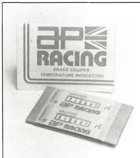
Temperature-indicating labels are for use on disc-brake calipers. Note the word CAUTION starting at 320F (160C). Temperature indicates fluid may be boiling inside caliper. Photo courtesy AP Racing.
