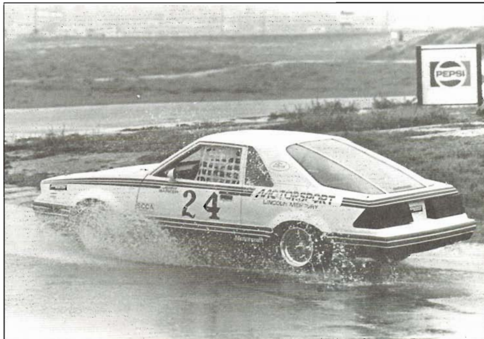
This Mercury requires adjustable brake balance for two reasons. Switching from street driving to racing increases weight transfer and requires more braking effort on the front wheels. Racing in the rain reduces weight transfer and requires less braking on the front wheels compared to racing in the dry. Photo by Steven Schnabel.
