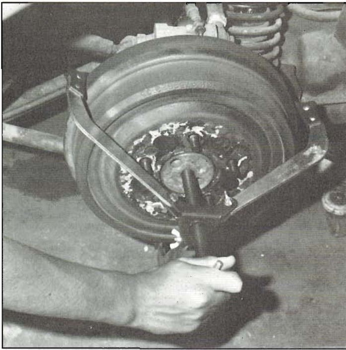
Special puller is designed to remove brake drums. Thin jaws grasp back of drum. Handle is then turned carefully by hand—not with a wrench or lever. Excess force will break or distort drum or puller. Tapping drum lightly with a plastic mallet is OK to assist removing a stubborn drum.
