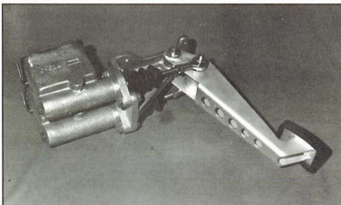
Dual master-cylinder setup manufactured by Neal Products, fitted with Howe cylinders, is popular for use in racing stock cars and other special vehicles. Hurst/Airheart, Girling or Lockheed master cylinders can be used with this setup.
