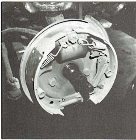
Typical duo-servo front brake used on large front-engine, rear-drive American cars; anchor pin is above wheel cylinder. Adjuster joins lower ends of shoes. Only rigid connection between backing plate and shoes is at anchor pin.
