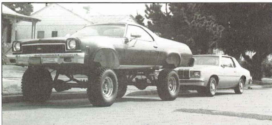
If you change CG height of a car, you need to change brake balance. A tall car has a greater weight transfer than one with a low CG. I hope the owner of this truck never has to stop fast from high speed—or has to do anything else at high speed.
