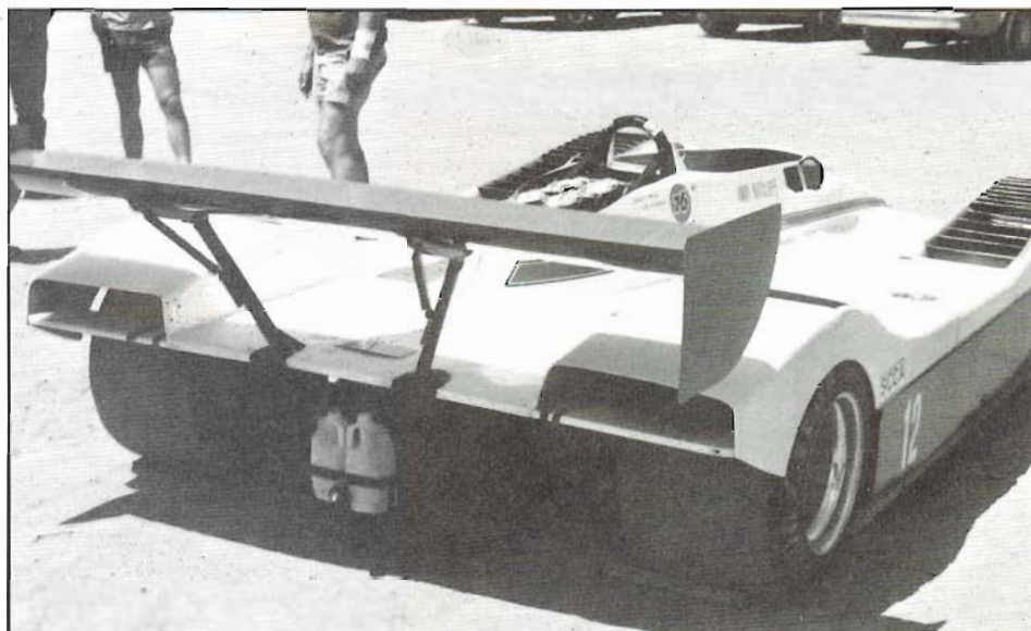
Wing at rear of sports racer improves rear-tire traction for improved handling and braking at high speed. As speed drops, so does wing downforce, increasing the chance of rear-wheel lockup when braking for tight corners.
