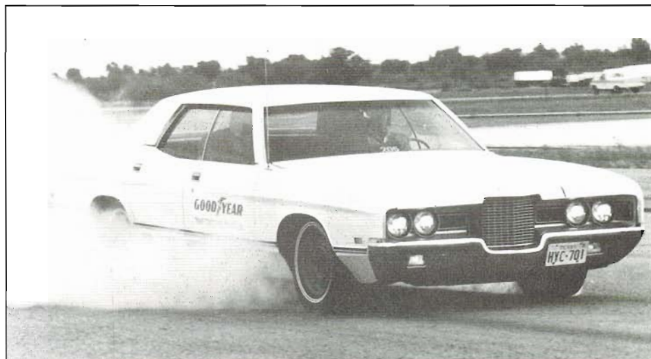
Tires on this car have reached their maximum coefficient of friction. Although a car stops faster if the wheels are not locked, most drivers hit the brakes too hard during a panic stop. This test, being conducted at Goodyear's San Angelo, Texas, test track, is to see how tires react during a panic stop. Photo courtesy Goodyear.
