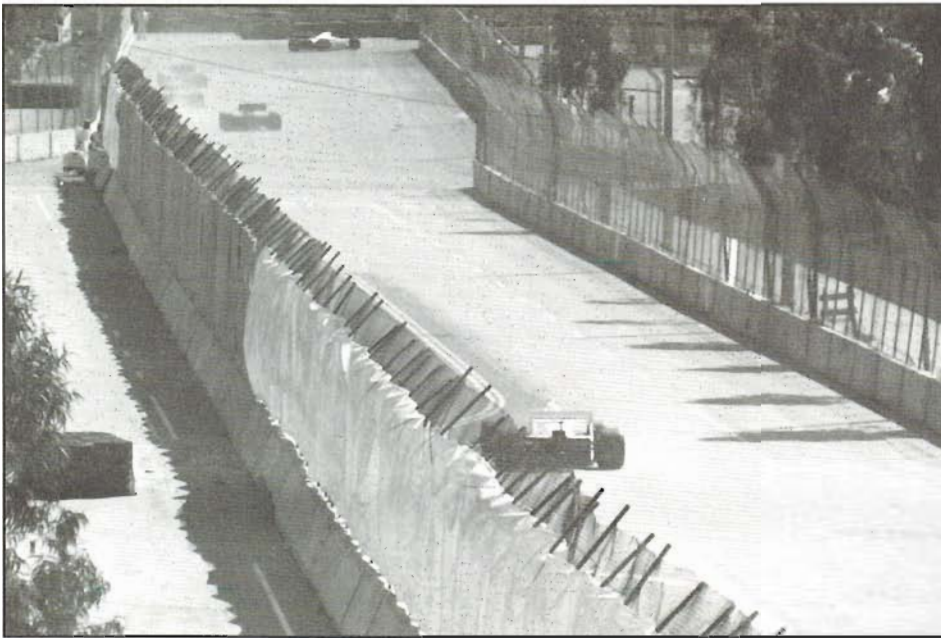
Grand Prix cars frequently run on courses with long straights and tight turns, which is extremely hard on brakes. Friction-material hardness is selected to match the course. "Hard" linings are required when running a race like this one on the streets of Long Beach.
