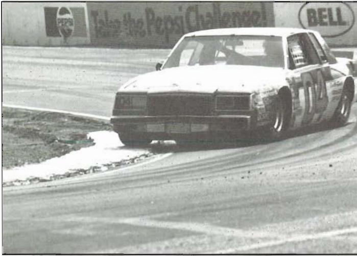
Maximum loads can occur in two directions at once. Here, stock-car driver cuts a close apex. Resulting bump load from going over curb on right front wheel occurs at same time as maximum cornering load.
