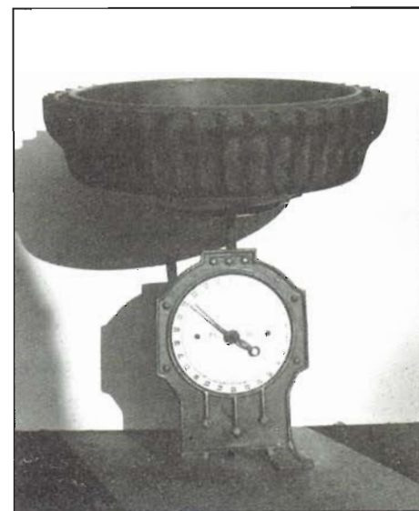
The heavier a drum or rotor, the lower its temperature rise during a single stop. Designed for a 3000-lb sports car powered by a 300-HP engine, this large drum weighs 22 lb.
