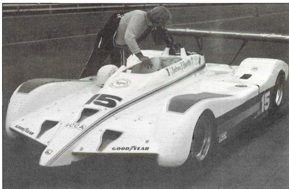
Ground effects and rear wing provide maximum aerodynamic downforce. Wing also increases drag dramatically. NACA ducts optimize airflow to brakes with minimum drag.
