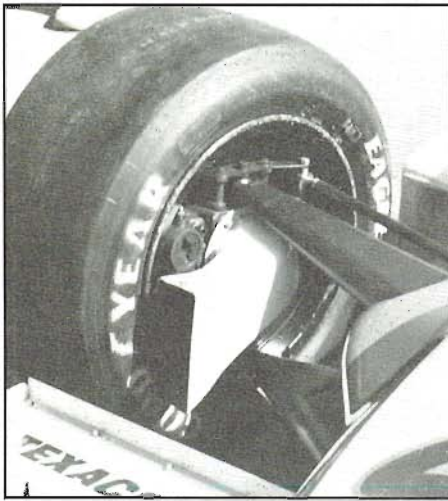
Fiberglass scoop on this Indy Car brake is sealed to front upright. Air is ducted directly to center of vented rotor. This duct was obviously designed with rest of the car, and not merely added on after brakes overheated. Photo by Tom Monroe.
