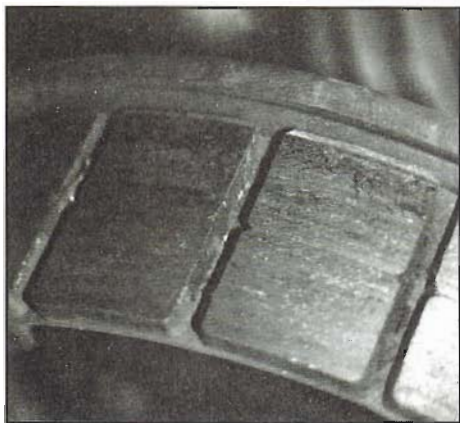
Metallic linings for 1962 Corvette drum brakes were highly successful for racing. Prior to the use of disc brakes, drum brakes with these linings were relatively fade-free, even on a 3000-lb, 300-HP sports car.
