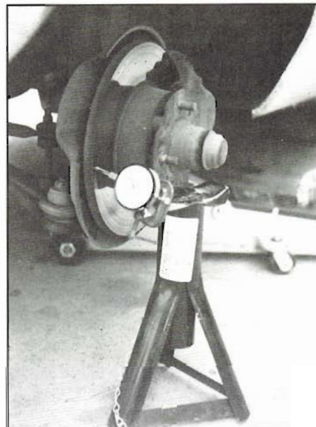
Checking rotor runout is done with dial indicator clamped to a jack stand. Runout of 0.005 in. is considered upper limit for most cars.
