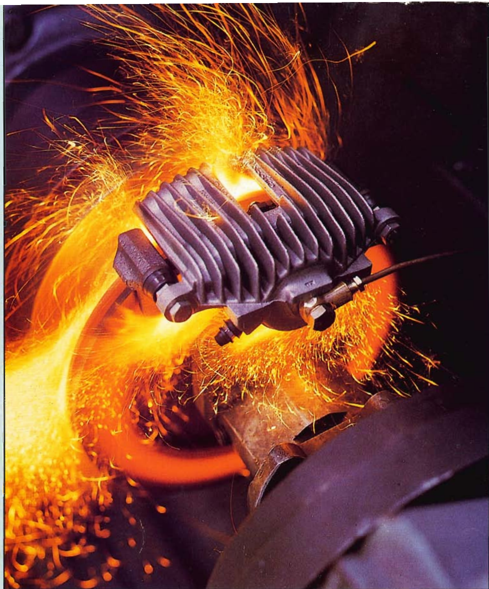
Corvette disc-brake pads being tested to destruction on Girlock dynamometer, page 105. Photo courtesy Girlock Ltd.
