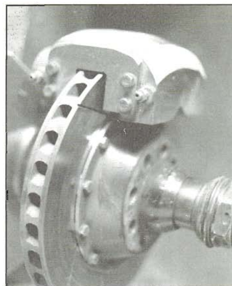
Caliper did not fit wheel correctly, so metal was removed from outboard edge. Don't do this to get a caliper to fit. Caliper flexing, cracking or other problems may result if excess metal is removed. Instead, select calipers and wheels that clear without modification.
