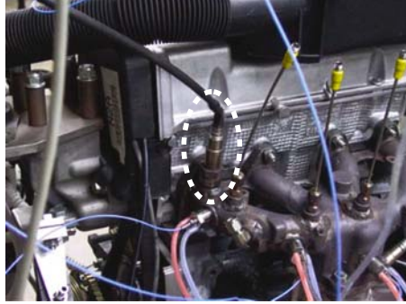
Fig. 7. Location of the UEGO sensor (dotted oval)
