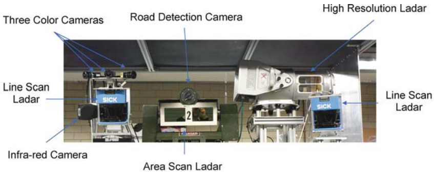
Fig. 4. Sensor suite mounted on the HMMWV cab
