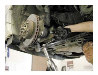
Step 8: Install the new balljoint — complete with grease fitting, rubber boot, castellated nut and cotter pin — using the hardware that came with it. Torque it to factory spec.
