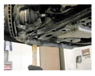
Step 7: Remove the balljoint, pulling down on the control arm for clearance if necessary.
