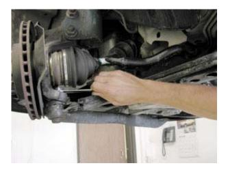
Step 4: Remove the old joint's cotter pin and castellated nut.
