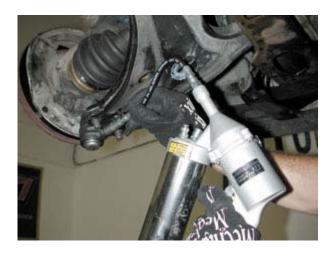
Step 9: Lube the balljoint, wiping off any grease that spews out around the boot.
