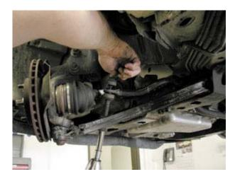
Step 3: Loosen the swaybar endlink (if applicable).
