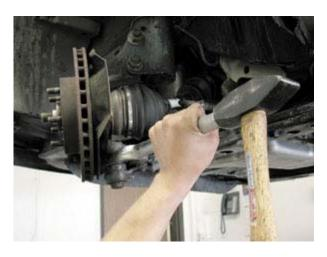
Step 5: Separate the balljoint using a prybar or pickle fork. Then loosely reinsert the stud in the knuckle.
