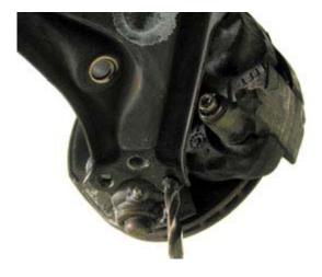
Step 6: Many shops use air chisels to remove balljoint rivets, but the do-it-yourselfer is better served with a drill. Service manuals normally give bit sizes appropriate for drilling out balljoint rivets without damaging the control arm.
