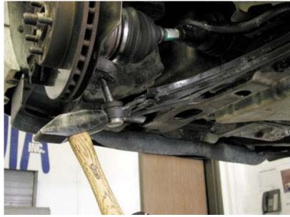
As people as diverse as Liz Taylor and Eddie Van Halen can attest, joints wear out. In cars, ball-in-socket joints degrade over time (similar to their human counterparts). Lack of lubrication and dirt inside moving parts will accelerate the demise of a vehicle's joints.
