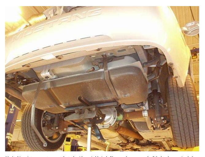
11. At this point you must support the tank with a suitable jack. You can then remove the 3 fuel tank mounting bolts. Install a safety chain or strap (not shown) to prevent the tank from slipping off the jack as you lower it. The tank must be simultaneously lowered and pushed to the driver's side of the car to allow the filler neck to clear the fill pipe grommet.
