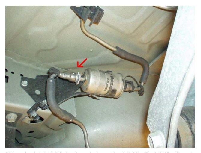
10. Shown above is the fuel feed line from the pump/sender assembly to the fuel filter. Note the fuel line release tool already installed. Remove the fuel line from the filter with the release tool.
