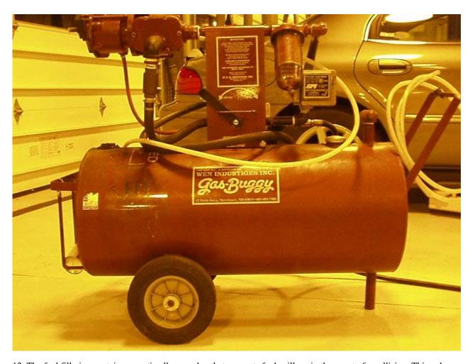
12. The fuel fill pipe contains an anti-rollover valve that prevents fuel spillage in the event of a collision. This valve also prevents removing the fuel from the tank when it is installed in the car. Once the tank is clear of the fill pipe, a hose can be inserted in to the fill pipe opening and the tank can be drained. We used a Gas Buggy for this purpose. DIYers can use a manual siphon pump and approved storage containers. **NEVER SYPHON BY MOUTH!**
