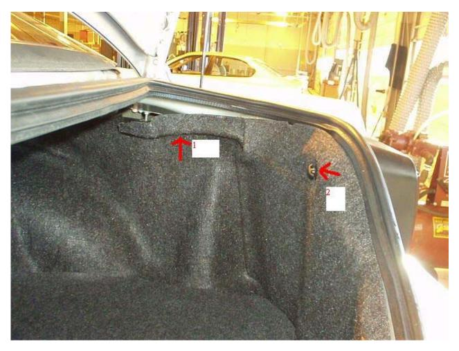
4. We then opened the trunk and removed the two trim panel retainers.
