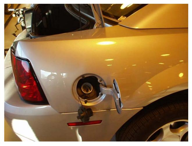
3. We removed the fuel cap and the 3 screws that secure the filler neck to the car's body.
