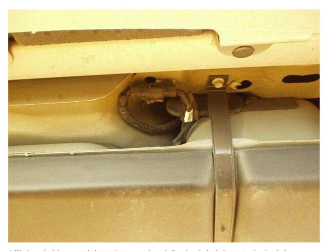
6. We then raised the car on a hoist to gain access to the tank. Seen here is the fuel pump/sender electrical connector. This connector must be disconnected and freed from the trunk floor.
