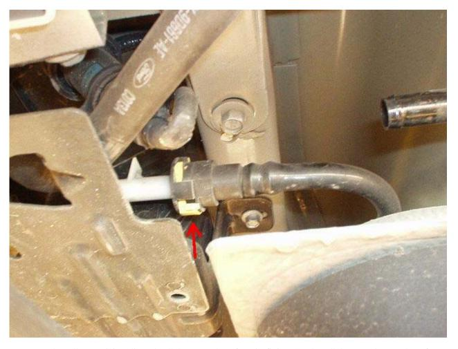
7. Depress the yellow retaining clip and pull the EVAP hose from its fitting. Gently pull the second EVAP hose from its fitting (seen here already disconnected).
