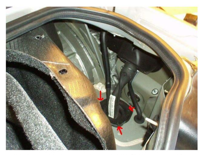
5. With the trim panels pulled back, we can access the 3 screws that hold the fill pipe grommet to the trunk floor. We remove these 3 screws to allow the fill pipe to drop down as the tank is lowered.
