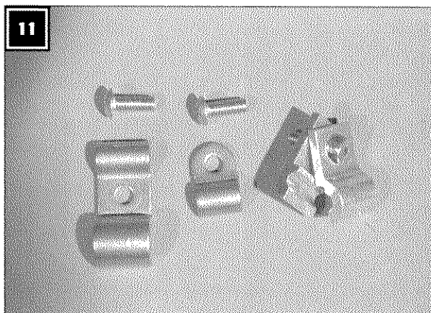
A variety of clamps are available to hold the line in place along the frame.
