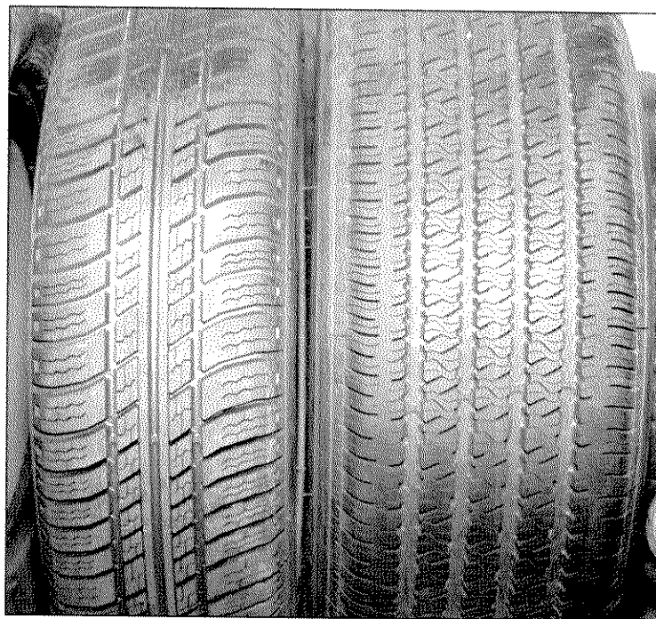
Two very similar tires, likely to have very different effects when driven in the rain. Note how the siping on the left-hand tire is designed to help the water exit from under the tire, while the tire on the right is likely to trap that same water.
