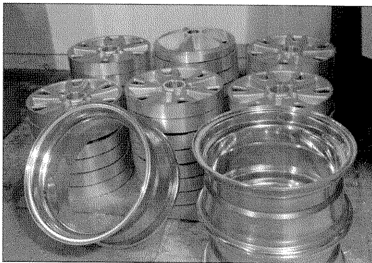
Though we think of billet wheels as being two-piece designs, these two-piece wheels use a cast center. This type of wheel makes it easier to provide a wide range of backspacing simply by changing the position of the center relative to the rim.
