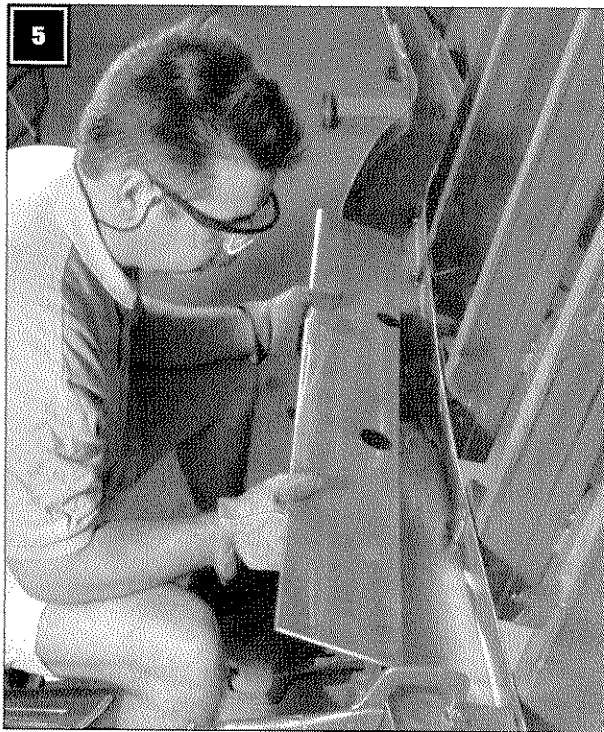
Each piece of the boxing plate is set in place and fit, then the three pieces are welded into one before being set back into the frame for the last time.
