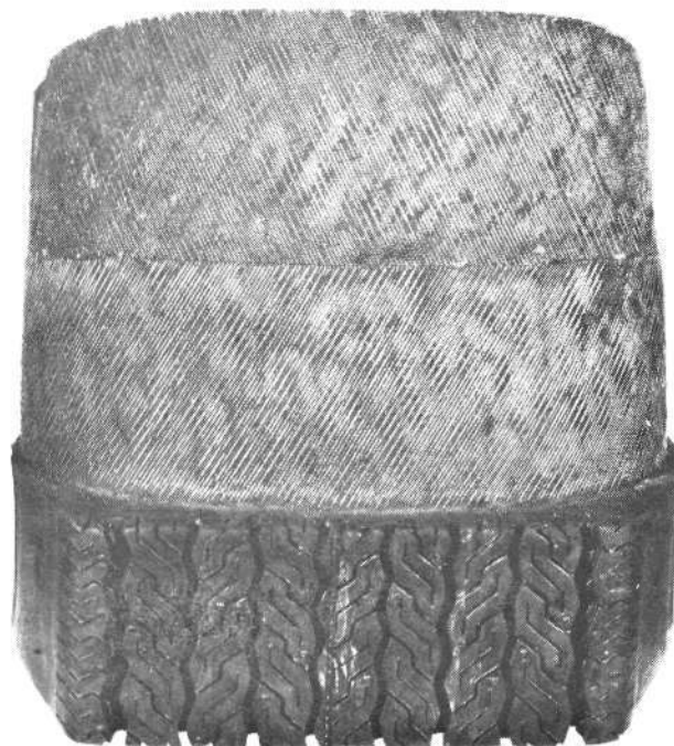
This is Firestone's Super Sports Wide Oval passenger tire. It is bias construction, two-ply nylon cord. This is a wide-tread tire, but shares the stiffness characteristics of all bias-ply tires. Notice the cord angles under the tread.
