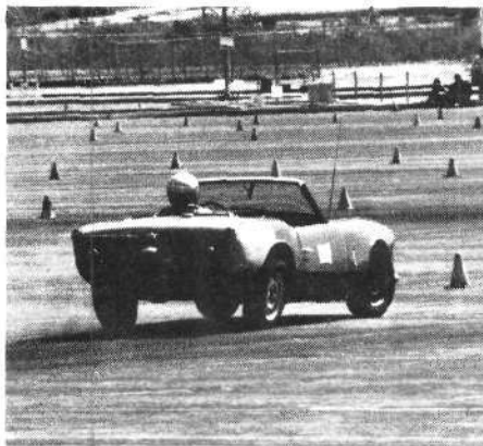
This early Spitfire is one of the poorest handling sports cars in stock form due to the swing-axle rear suspension. Jacking effect in a turn causes the car to thrust its tail upwards like a stink bug. The result is a large amount of positive camber on both rear tires and lost traction. Late model Spitfires have greatly improved rear suspension.
