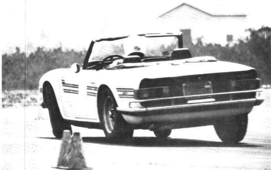
This stock Triumph shows a lot of body roll in this slalom turn. Notice the large amount of positive camber on both outside tires, particularly the front. This car is strongly understeering, and just from looking at the photo it seems mostly due to this camber change. This car would corner faster and probably understeer less if roll stiffness were increased.
