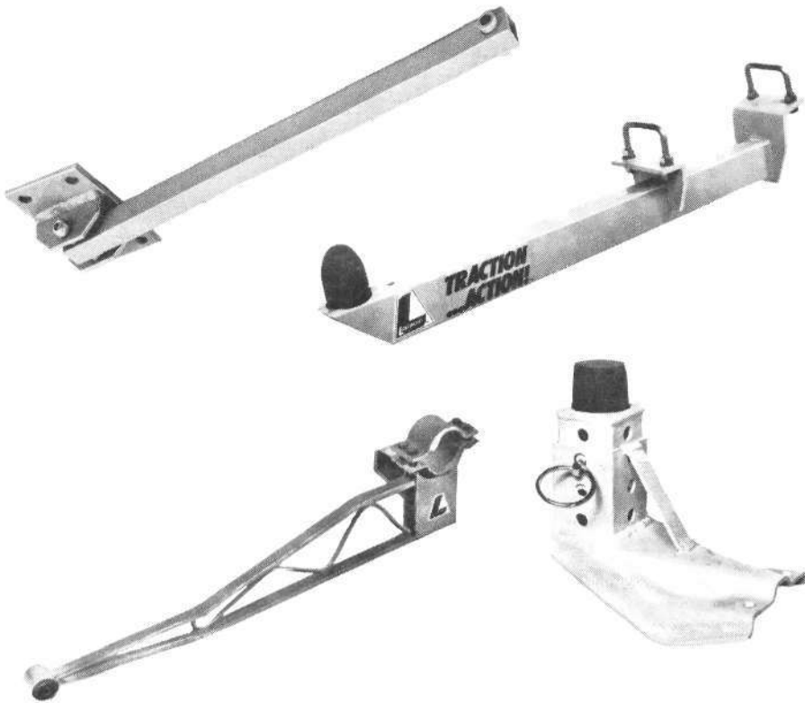
Here are some products for drag racing manufactured by Lakewood Industries. Lower left is a lift bar with a pivot at the forward end. The lift bar at the upper right uses a rubber pad rather than a pivot, so it will be more suitable for cornering. Upper left is a traction bar, this particular one used on a Corvette. Lower right shows a pinion snubber to fit a Chrysler Corporation axle housing. (Photos courtesy Lakewood Industries)
