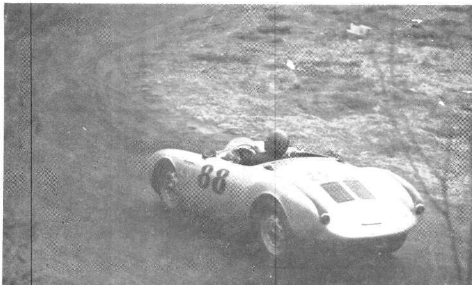
A critical part of a turn is the instant when the driver first starts to turn the wheel. The car's transitional handling characteristics describe what happens at this instant between going straight and turning. This is very complex and sensitive to many factors in chassis design and adjustment. (Chuck Engberg photo.)
