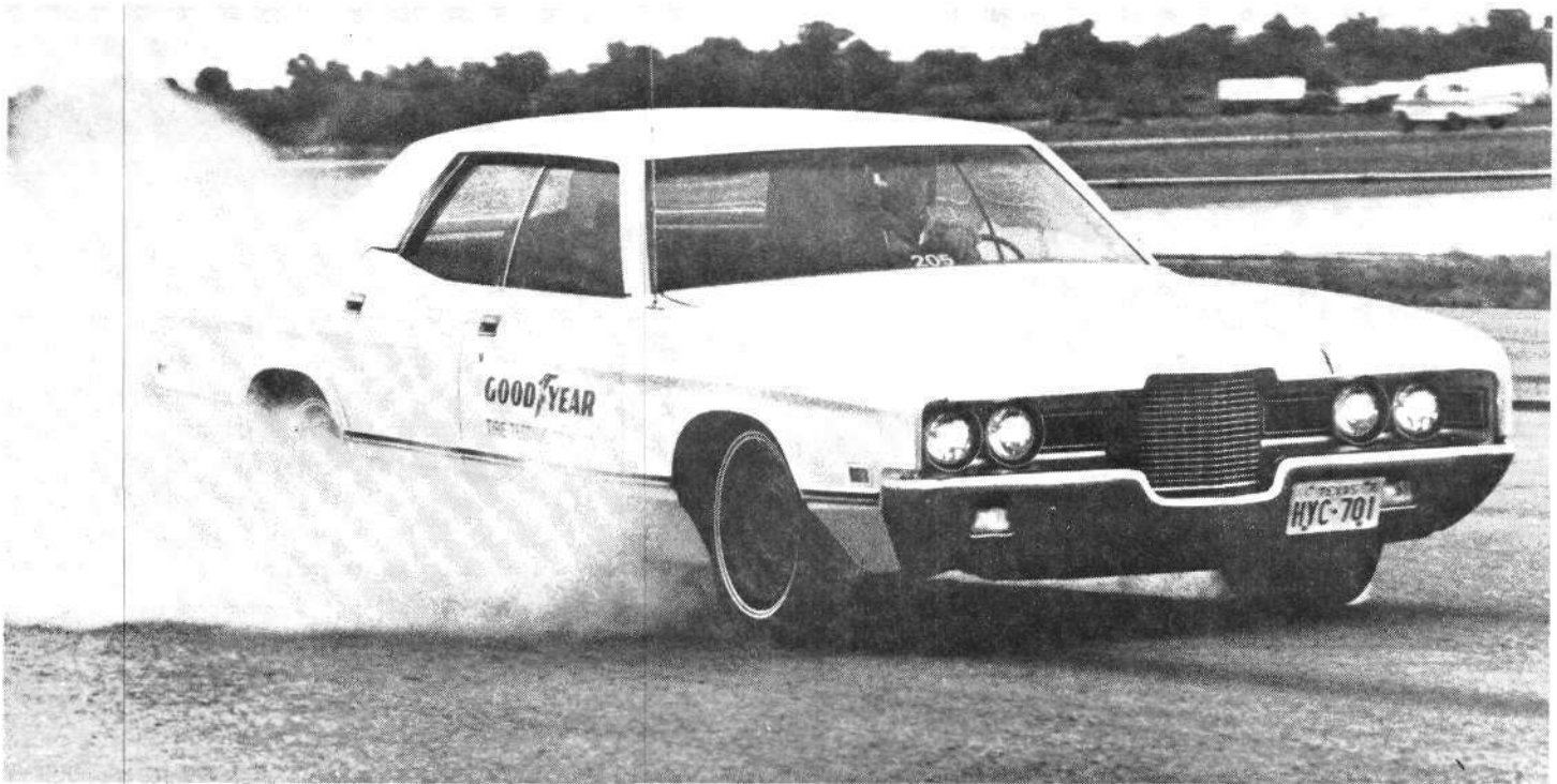
Driver is locking the front tires in a braking test at the Goodyear San Angelo Texas proving ground. Testing brakes in this manner can quickly destroy the tires, so take it easy. (Photo courtesy Goodyear Tire & Rubber Co.)
