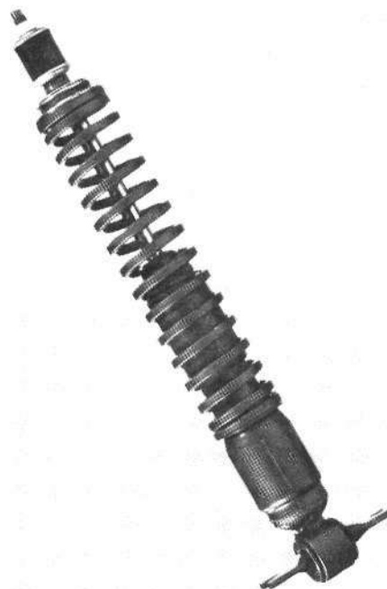
This Monroe Load-Leveler is both a heavy-duty shock absorber and an auxiliary coil spring which adds to the suspension stiffness. Although it has both a spring and a shock, these units are not intended to serve as the entire suspension. (Photo courtesy Monroe Auto Equipment Company)
