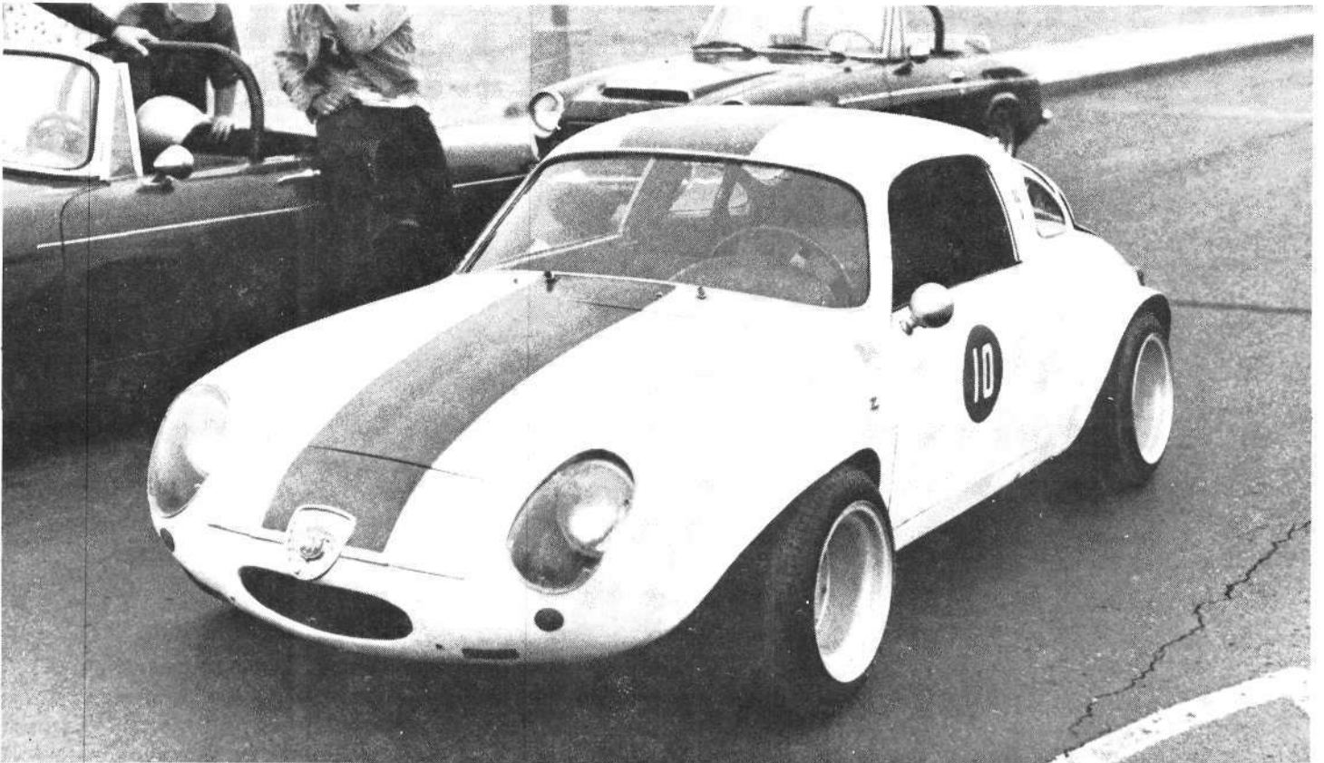
This Fiat Abarth started life as a fun little road car that gave lively performance, good handling, and reasonable practicality. After owner Chuck Thompson's modifications it was a fire-breathing monster, impossible to drive on the road, but capable of winning top-time-of-the-day at slaloms. This little car with its Formula One slicks and rock solid suspension consistently beats Corvettes and Cobras due to its superior handling.
