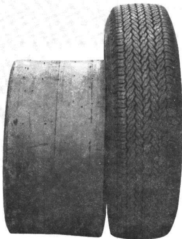
A modern racing tire and a radial street tire are shown for size comparison. Both tires fit a Datsun 510 sedan and use a 13" diameter wheel. The racing tire will give about 50% more traction than the street tire on dry pavement, but the street tire is superior in the wet. Unless you are racing in the dry, stay away from the slicks.
