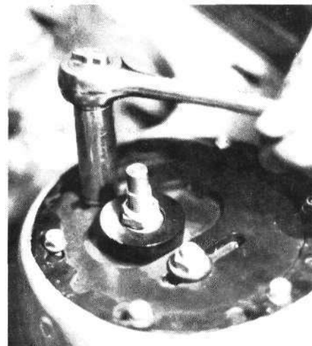
This Datsun has MacPherson-strut suspension with a modification. The camber is adjustable by means of sliding the top end of the shock strut in the slots shown. The mounting bolts are being loosened prior to making the camber adjustment. Normally these cars do not have a camber adjustment.
