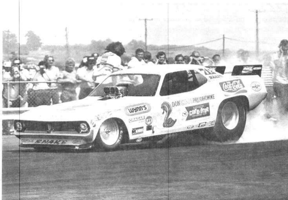
Drag racing tires are brought up to racing temperatures with a burnout before a run. Here Don Prudhomme heats the tires of his funny car. The tires are deliberately allowed to break traction by pouring liquid bleach in front of them before the driver gets off the throttle. (Photo courtesy of Cragar Industries.)
