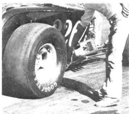
Pit crew member pours liquid on the pavement in front of the rear tires prior to a burnout. Wheelspin in the burnout heats the tires so they get maximum traction during the race. The tires must remain hot to be effective.
