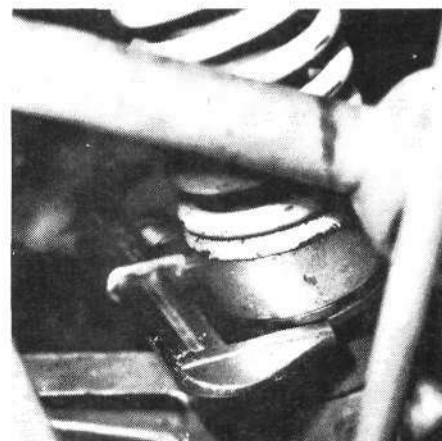
Before measuring ride height take the friction out of the suspension by bouncing it as shown. On some cars the only way to get accurate ride height measurements is to remove the shocks.
