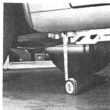
A convenient place to measure the ride height of the 1975 Pinto is under the rocker panel just in front of the rear wheel. There is a convenient flat surface on the bottom of the body at this location. It's easy to see the scale without having to crawl under the car. This car has a ride height of 9 inches. Notice the muffler in the background is closer to the road.
