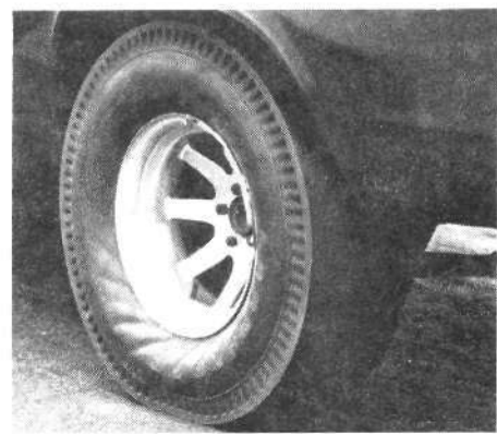
This sedan is typical of a drag-race car that is also driven on the street. It is raised up for improved weight transfer, and drag slicks are installed for the race. Notice the large contact patch of this low-pressure tire. The car is accelerating without wheelspin, and the torque wrinkles the sidewalls of the tire.
