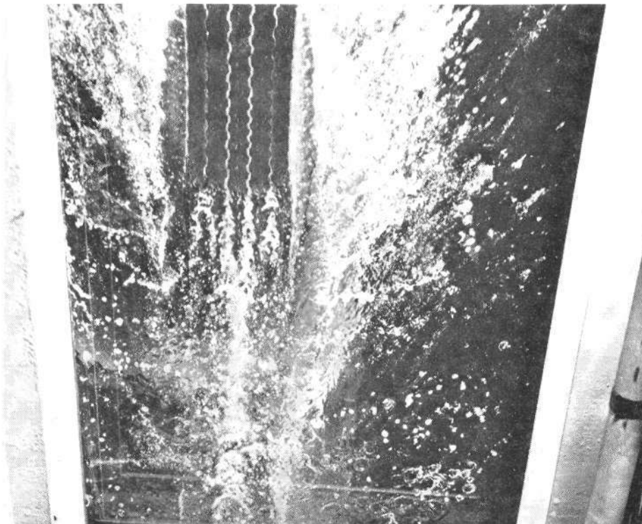
Engineers can observe and photograph tire behavior through a glass plate set into the test track at the Goodyear proving ground near San Angelo, TX. Photographs of tread distortion and hydroplaning are analyzed to help design tires with improved performance. (Photo courtesy of Goodyear Tire and Rubber Co.)
