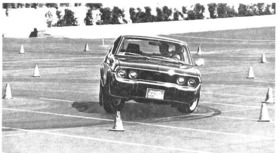
This stock Mazda comes with severe understeer in tight turns. In this slalom the car is close to hitting the cone in front of the car even though the driver has the steering near full lock. Understeer is safe for your grandmother, but it isn't the quickest way around a race course.
