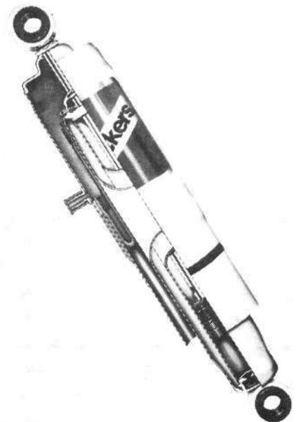
Air-adjustable shock absorbers are pressurized air in a cavity inside the shock to add stiffness to the suspension—just as an added coil spring does. This cross-section of a Gabriel Hi-Jacker shows the air valve and a flexible diaphragm which converts the top portion of the shock body into an air chamber. (Photo courtesy Maremont Corporation)
