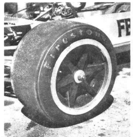
Front wheels of March Formula car have negative offset. This puts steering pivot axis near center of tire for easier steering and better handling.
