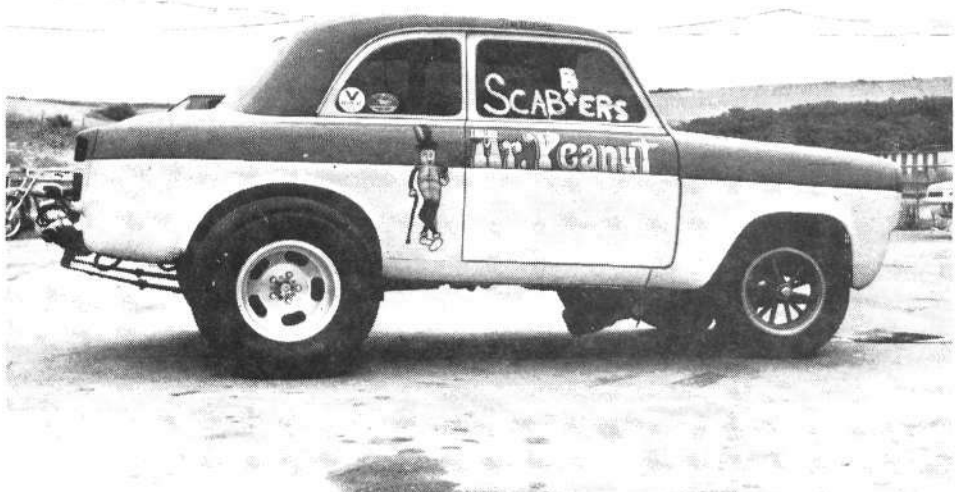
The tires on a typical drag-racing car are narrow and light on the front and huge on the rear. The rear tires are light too, but put a very large contact patch on the ground. This car uses special magnesium wheels on the front, suitable for drag racing only.
