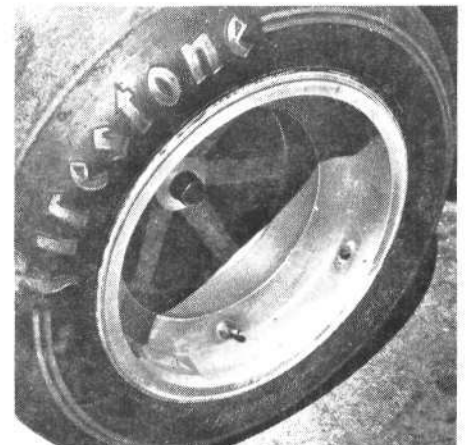
Rear wheels on this March Formula car have positive offset to reduce loads on the wheel center and wheel bearings during hard cornering. This is explained in Figure 35.
