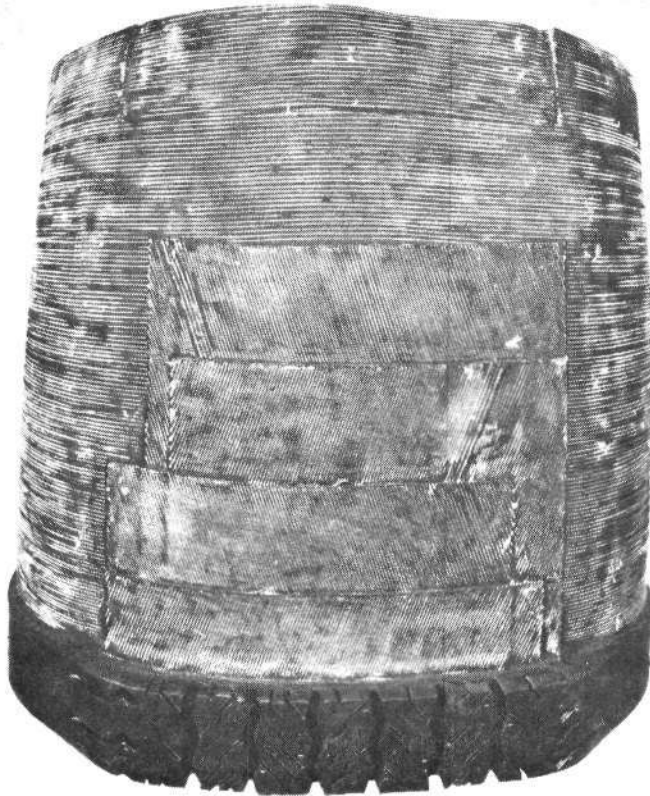
Here's a close-up of the interior construction of Firestone's Wide Oval Radial passenger tire. It has two radial body plies and four belt plies. The belt material is criss-crossed for maximum lateral stiffness, and the 90-degree cord angle of the sidewalls allows flexibility.
