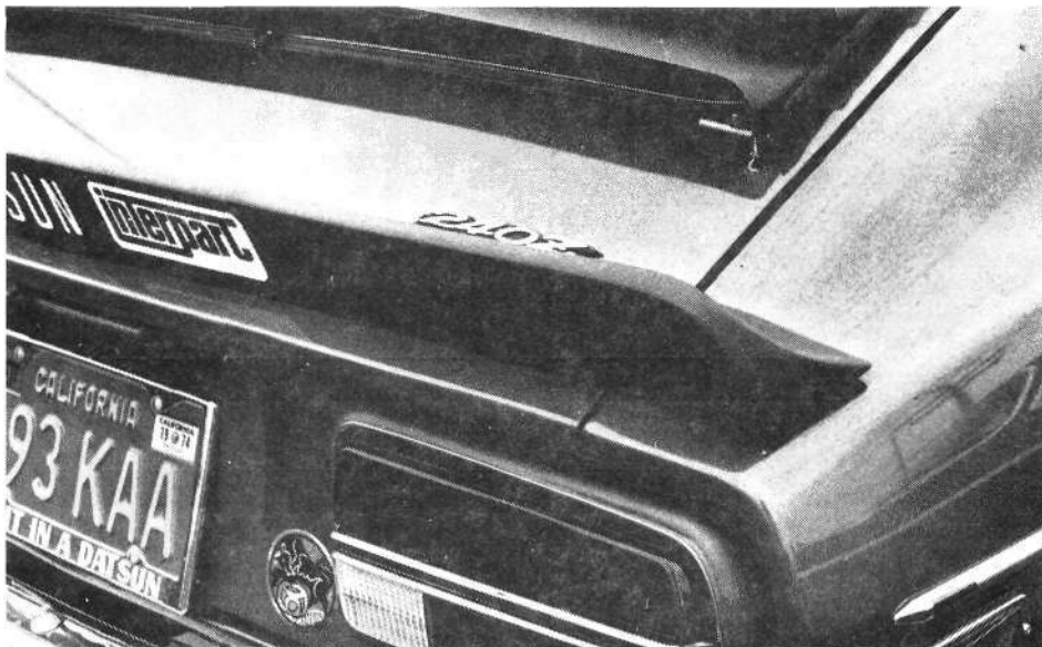
This fiberglass rear spoiler is an accessory. It is just for looks at legal highway speeds, as it is too small for the weight of the car. Also the air tends to separate off the roof and ruin the flow that hits the spoiler.
