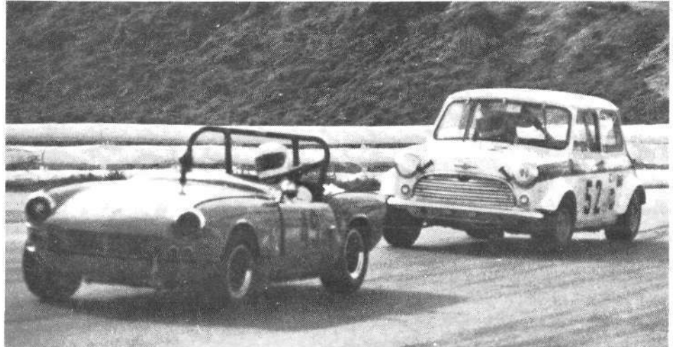
Ron Moore selected a right-hand drive Mini for road racing to have an advantage in right-hand turns. Here at Riverside Raceway, where he does most of his racing, there are more right turns than left. At this point in a hard right turn he is able to apply power, where a left-hand drive car would have to wait an instant later before accelerating out of the turn. This works against him in left-hand turns.
