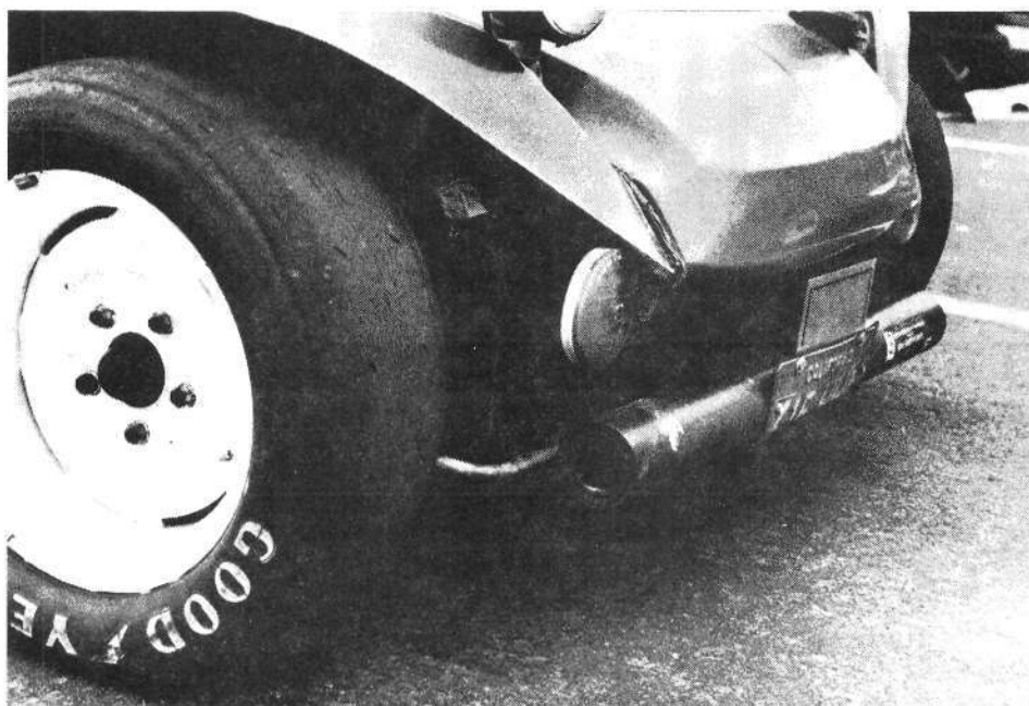
The owner of this slalom buggy felt a need for more weight on the front tires so he installed this ballast as a front bumper. Usually a handling problem can be cured by more efficient means, but if the CG has to be moved this is one way to do it.
