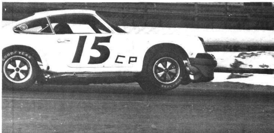
This Porsche has been set up with too much roll stiffness in the front suspension, and the front tire is lifting off the road. The car would corner flatter if more roll stiffness were added to the rear suspension—and cornering speed would be improved.
