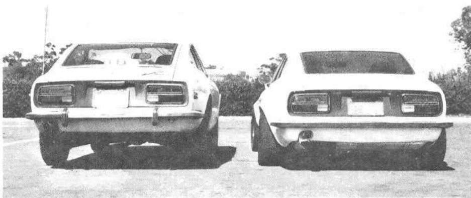
Here's what can be done in an all-out effort to get better handling on the street. The Datsun on the right belongs to George Louis of San Diego. Besides the obvious lowering of ride height, the car has many hidden improvements: Interpart Mulholland springs on Koni shocks, 23mm anti-roll bar front and rear, Goodrich 50-series radial TA tires on 13 x 7 mag wheels. Solid bushings are used in the suspension pivots. Mitchell steering rack in stiffer rack-mounting bushings gives quicker steering response. Stopping is improved with Velvetouch brake linings, steel braided brake hoses. Brake cooling ducts are in the front spoiler. This car is an ultimate street machine, and is only slightly illegal in California. A stock Datsun is shown on the left.
