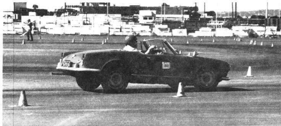
This Alfa is braking hard for a corner. You can see the nosedive resulting from forward weight transfer. The front brakes take most of the heat on this car because the front tires do most of the stopping.
