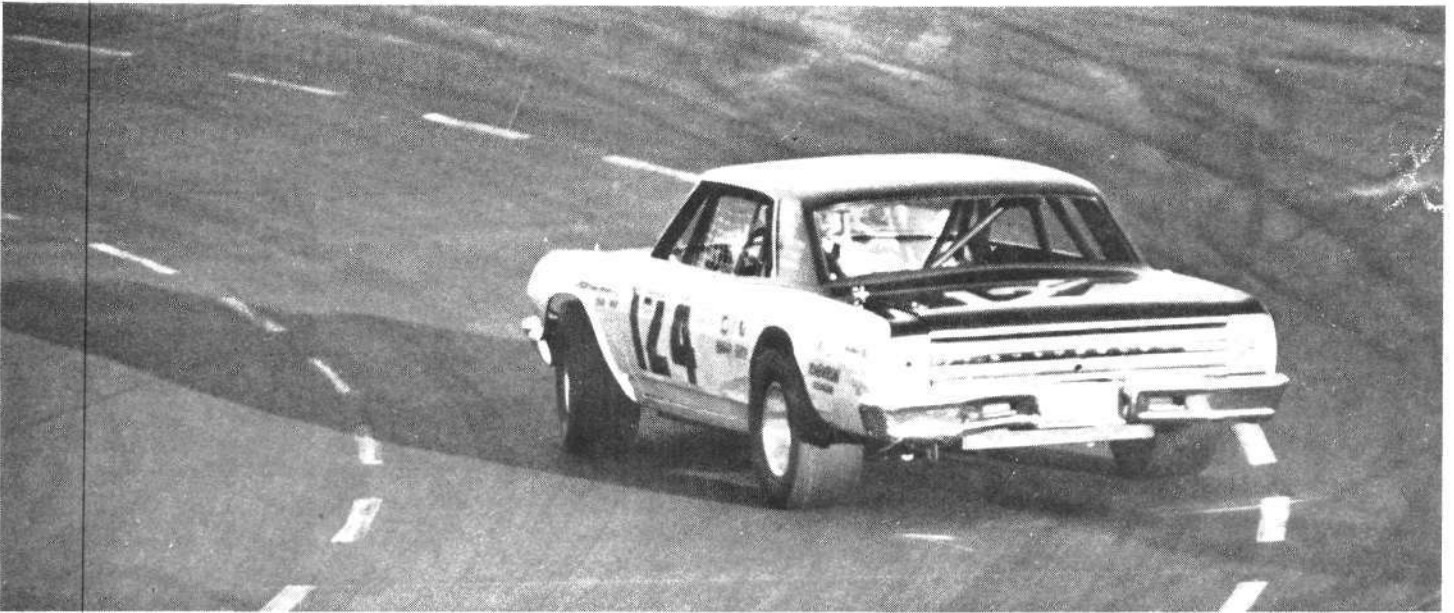
This car is using power coming out of a turn and is in an extreme oversteering attitude. Notice the front wheels are turned to the right even though this is a left hand corner. If the driver backed off on the power the car would straighten out, but he would have to do it very gently to avoid losing control.
