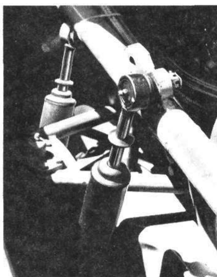
The rubber washer on the shaft on this shock is a suspension-travel indicator. The washer is pushed down against the shock body in the pits and its final position shows the amount of suspension travel after a run. These shocks are on a NASCAR stock car which runs on some steeply banked tracks.
