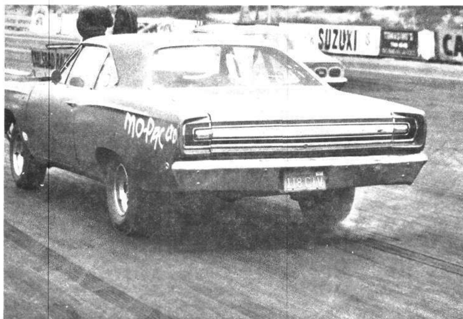
Here is what happens when you try accelerating hard with a stock car using a solid rear axle. The right tire breaks loose before the left one, reducing the maximum possible traction. Jacking the weight to add vertical load to the right rear tire will give better performance at the drag strip.
