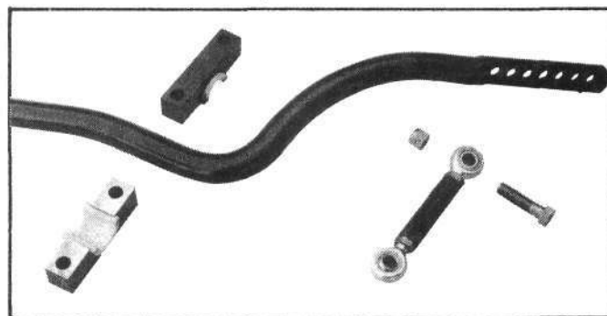
These sway-bars are modified production Chevette units. Solid bearings with Delrin inserts replace the production rubber bushings at the frame. The rear bar shown on the left uses an infinitely adjustable block with a weld-on round extension. The front bar uses an extension with a series of positive locating holes. This is due to the tight clearances at the front suspension.
