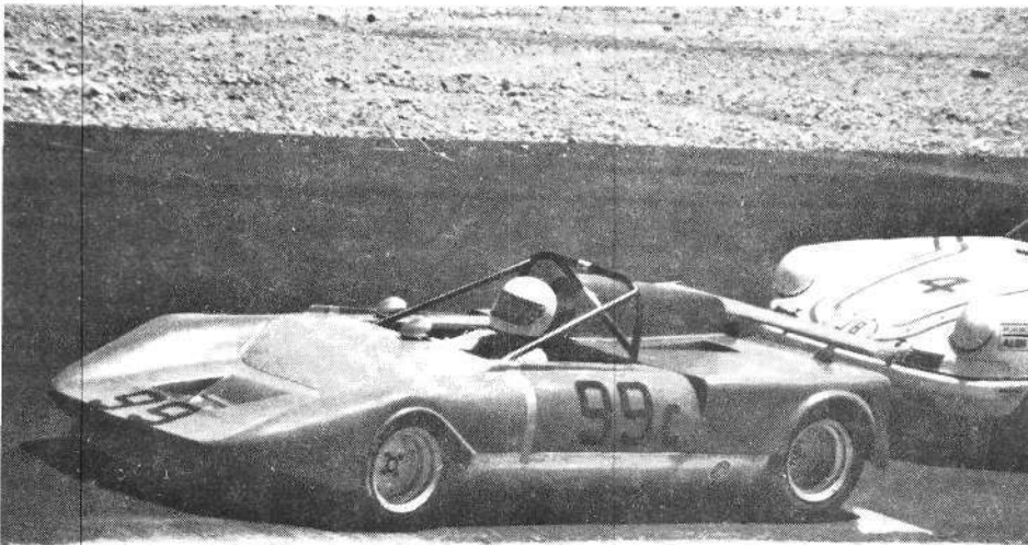
The low profile front tires on Rich Amick's Quasar allow a smooth air flow over the fenders. Larger front tires would seriously affect the air flow all the way back to the rear wing, plus would add frontal area. This small sports racer—designed by the author—will attain speeds of 140 MPH with only about 100 horsepower, due to the low-drag body. The body design was based entirely on the tire sizes.
