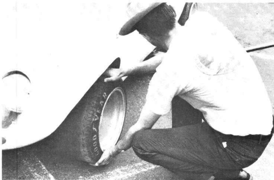
Play in the upper and lower suspension pivots is checked by attempting to move the tire in a camber direction. Play in this direction could be in either the steering pivots or in the suspension linkage pivots on the frame. Loose wheel bearings will also be noticeable with this test.
