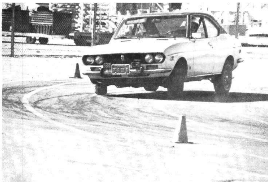
If you can get the use of a parking lot you can set up a small test corner using rubber cones or cardboard boxes for markers. On this lot the circular marks can also be used as a skid pad as described later.
