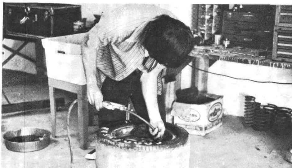
Racing mechanic Dave Mundy prepares for suspension tuning by balancing each tire and inflating to the usual operating pressure. Both are critical and should be checked frequently. The balancing tool used here is a simple static balancer. This works, but a more precise job is dynamically balancing by spinning the tires either on the car or on a wheel-balancing machine.
