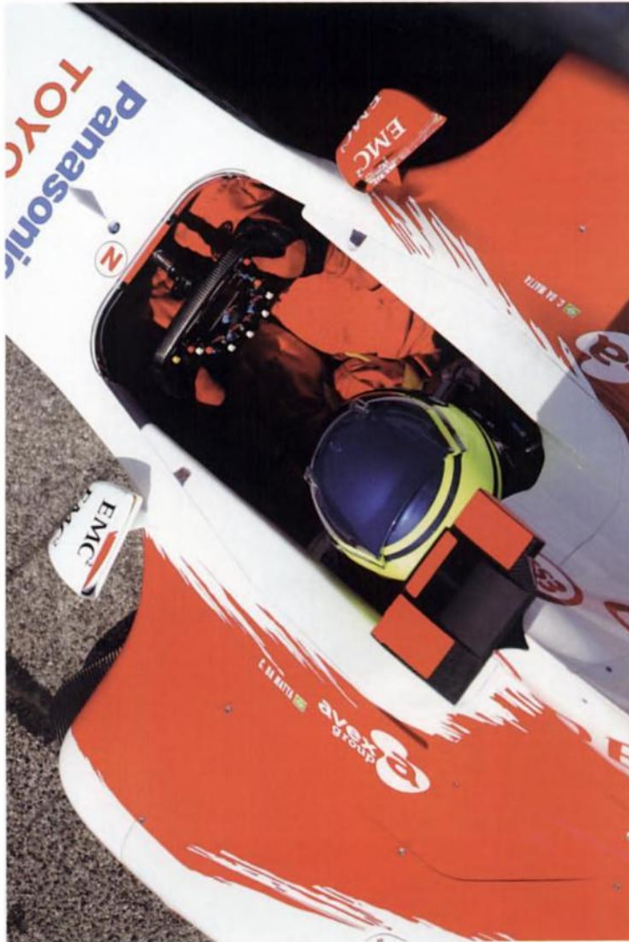
Plate 10. The original John Barnard designed 'paddle gear change system', as used today in all Formula 1 cars, is clearly seen being operated by a Toyota driver on today's state of the art steering wheel.
