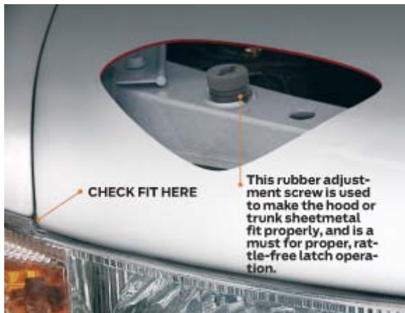
This rubber adjustment screw is used to make the hood or trunk sheetmetal fit properly, and is a must for proper, rattle-free latch operation.
