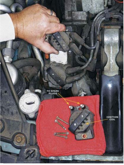
Swapping ignition coils in the coil pack of this GM minivan will tell us if one particular coil is the culprit. If it is, the misfire will move to a different cylinder.
