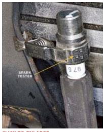
CLICK TO ENLARGE Spark testers are a safe way to see if coil output is up to snuff.
