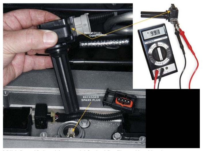
Individual coils mounted directly on each plug are easy to check. Secondary windings will have several thousand ohms resistance.
