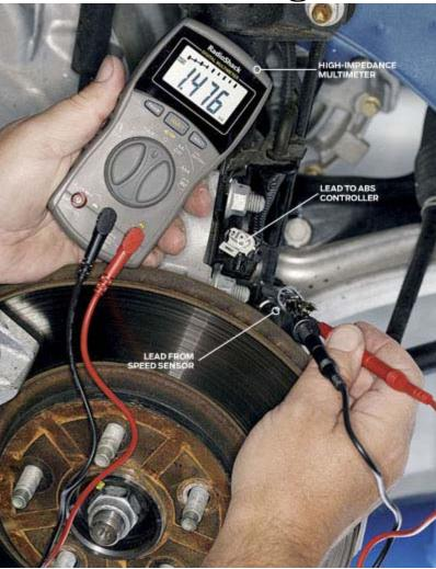
**Use your trusty multimeter** to check continuity through wheel speed sensors. This sensor has a value of about 1.5 K ohms.
