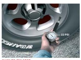
PSSST!: Low tire pressure will cause a wheel to pull.
