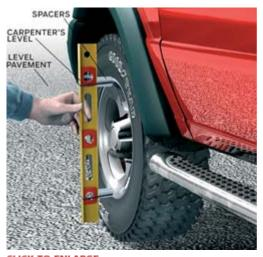
THIS SIDE UP: A quick camber check can be done with a level and two simple spacers.
