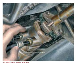
LOST MOTION: A deteriorated rag joint disc can cause slop in the steering.
