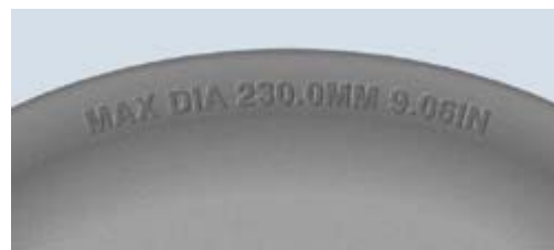
Brake drums will be marked clearly as to how far they can be machined safely to remove out of round.
