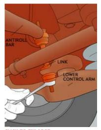
The antiroll bar's attaching links can become loose. Check the bushings.
