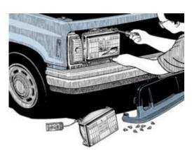
Replacing a broken headlamp assembly is straightforward. Most of the fasteners and mounting hardware will have to be transferred to the new
