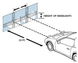
It's critical to keep both headlight beams' cutoff below the line at the bulbs' height from the pavement. Check this on level pavement.
