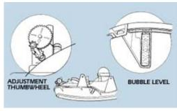
Many modern headlamp assemblies have a bubble level to assist in aiming the light beam. You'll still need a marked wall to see the beam pattern.
