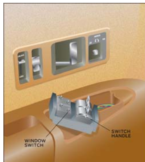
BOX OF SPARKS: If the fuse is okay, it's time to check the rocker switch assembly.
