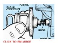
Pull the idle speed controller out of its bore to inspect the pintle tip, spring and air channel.
