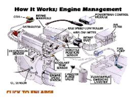
An automotive computerized engine-management system works like any computer as it controls idle speed. The central processing unit relies on various inputs to calculate necessary outputs. On modern motors, however, the inputs to the processor, or powertrain control module (PCM), are called sensors. The outputs are called actuators. And the PCM is programmed to control the actuators under any condition that the sensors deem necessary.
