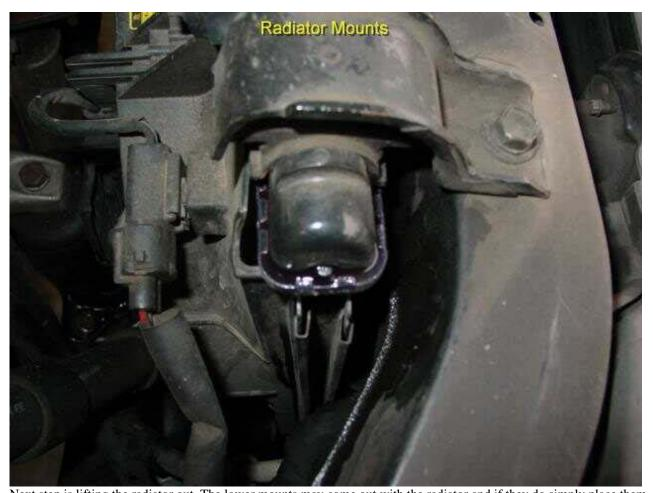
Next step is lifting the radiator out. The lower mounts may come out with the radiator and if they do simply place them back in the radiator support. I went a bit further and cleaned the A/c condenser by flushing all the bugs, dirt and road debris from it. You can do this with a garden or air hose to clean it. Air has to flow thru the condenser before it gets to the radiator so you are not only improving the A/c operation but the engine cooling as well
