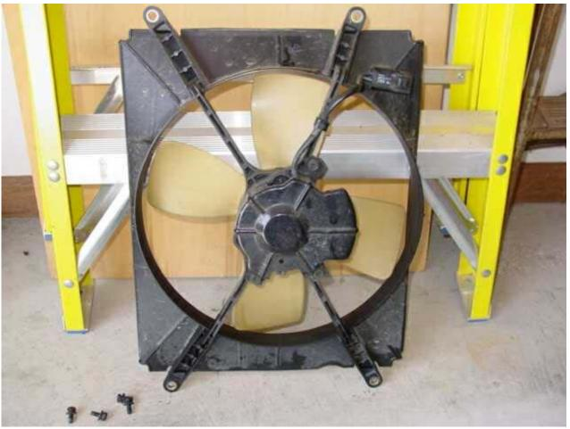
Nothing to it, four, 10mm bolts removed and the fan assembly is out of the way.
