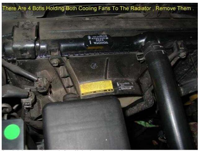
Once the bolts are out of the way the fan and its housing can be removed.
