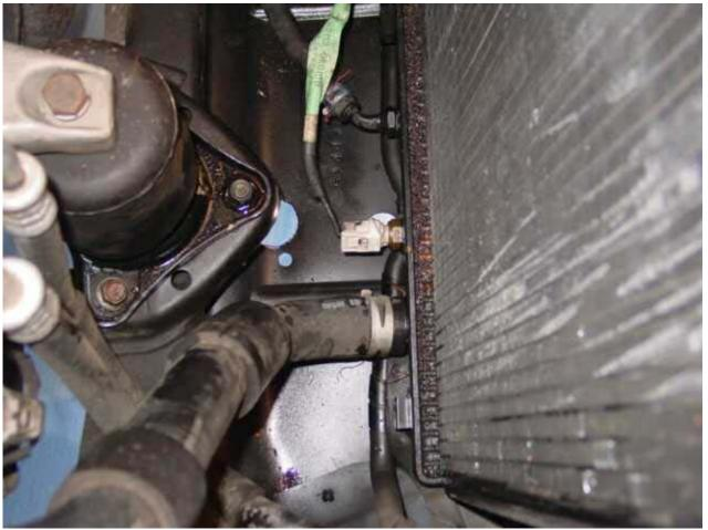
Once those are disconnected, the only thing holding the radiator in place is radiator mounting brackets, they can be removed with a 12mm socket and ratchet
