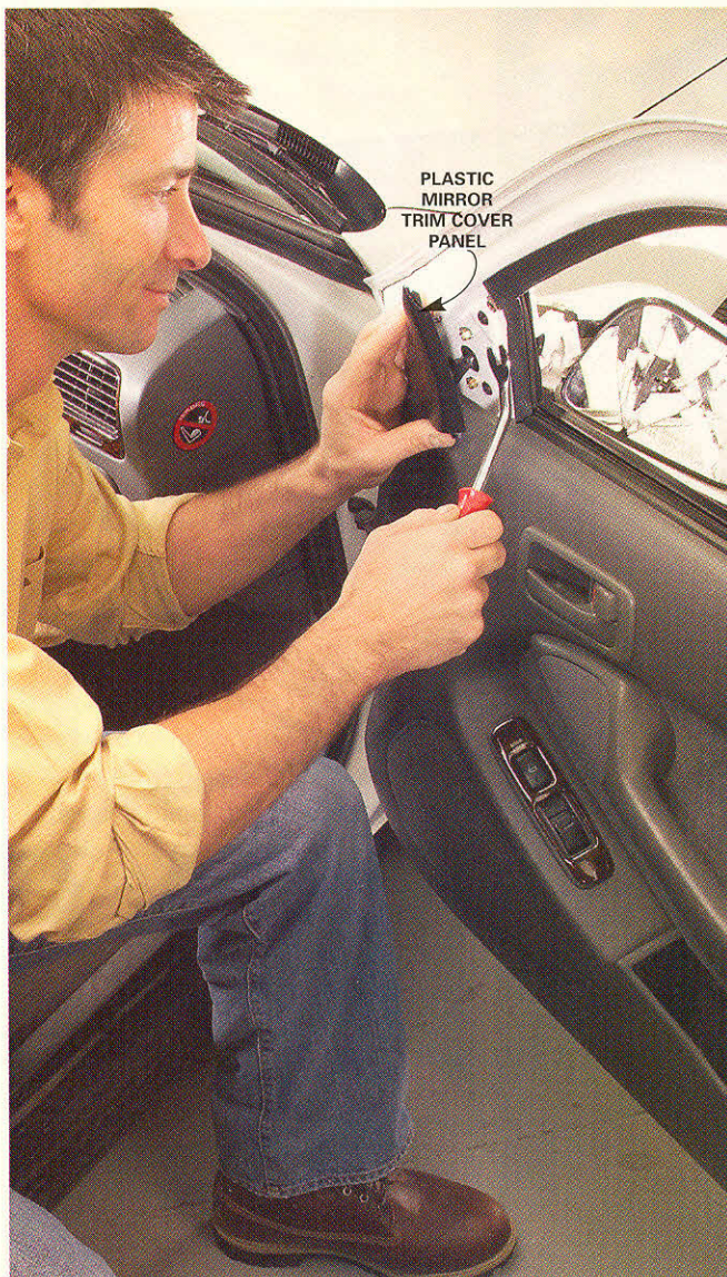
1 Pop off the mirror trim panel using the Door Panel Remover tool.
