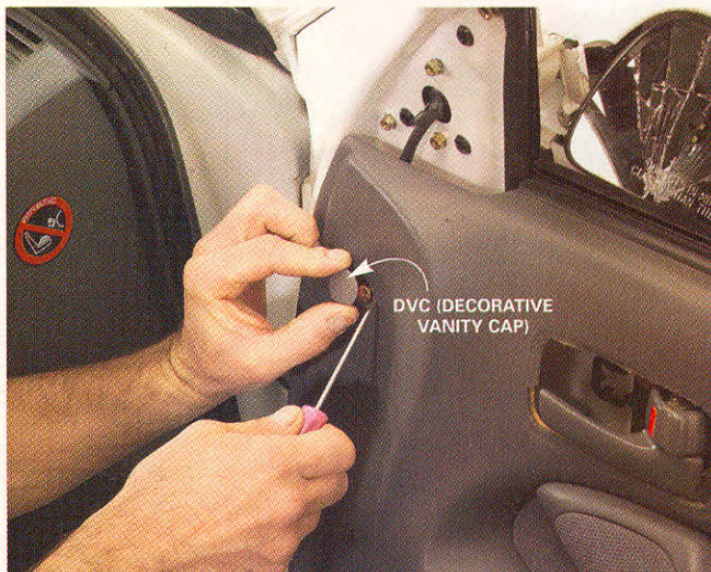
2 Remove decorative vanity caps from screws with the hooked pick, then remove the screws.
