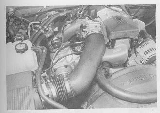
Everything is designed to fit in the stock engine compartment, and the entire kit can be installed using standard hand tools. A 5.3-liter kit consists of less than 10 components, not counting clips, clamps, and fasteners.
