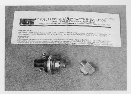
A number of protective options, such as this fuel pressure safety switch, can prevent a catastrophic failure. This switch will shut the system down in the event the fuel pressure drops below a safe level.
