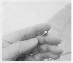
The tapered end of the jet seals against a flared tube. A scratch or nick in this area could cause a leak.
