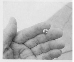
In this example, the orifice is a .028-inch hole.
