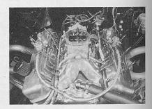
Nitrous oxide and fuel are transferred from their respective reservoirs to the solenoid valves through high-pressure braided steel hoses. These hoses are specific for nitrous oxide applications and contain a Teflon-coated inner tube. It is important these lines do not come into contact with any heat source, sharp edges, vibrating components, or parts that may squash them.
