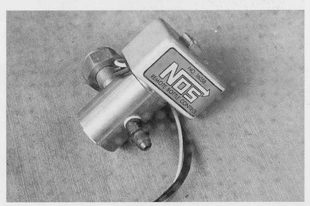
A solenoid-operated bottle valve can be wired for convenience, for safety, or both.
