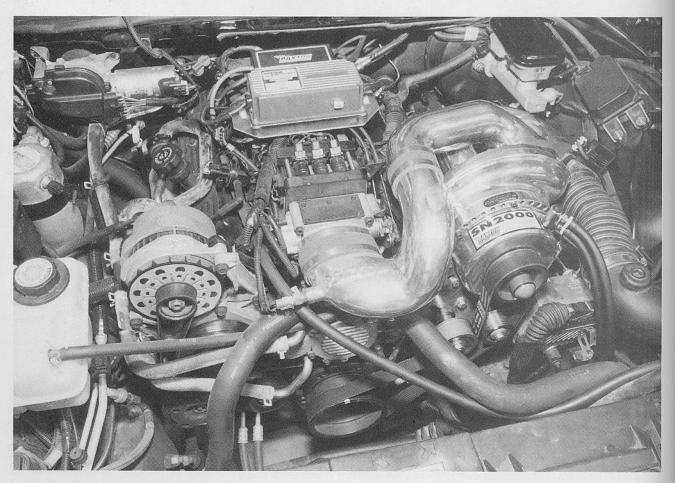
Paxton's 1101109-M and 1101112-M Chevy Impala SS kits exemplify modern forced induction engineering at its best. Paxton designed these kits around the super-quiet SN 2000 supercharger. A LT1 will generate 40 percent more horsepower on 92-octane pump gas when stimulated with 5 pounds of boost.
