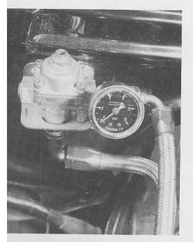
The stand-alone nitrous system has its own pressure regulator. The electric fuel pump servicing the nitrous system is activated only on demand. Always set the regulator to the flowing fuel pressure rate, not the static rate. In this application, the fuel supply system for the engine does not require a regulator.
