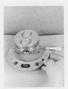
Pistons are barrel shaped, making it necessary to take several measurements perpendicular to the wrist pin halfway from the crown to the skirt. Use the largest measurement to set piston-to-wall clearance. Measure all of the pistons, then finish-hone each cylinder to allow for the blueprinted tolerance.
