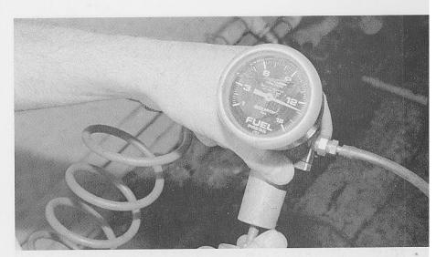
Using a compressed air source to simulate boost is a fast, efficient way to "dial in" a Super FMU baseline. Use an adjustable air pressure regulator to pressurize the manifold sensor port on the FMU in one-pound increments, then activate the fuel pump(s) to obtain a fuel pressure reading.
