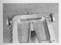
The bypass portal is cast into the blower housing to simplify packaging and ensure durability. The actuator can be mounted on either side of the blower and indexed in one of 12 possible locations (6 per side) around the shaft.
