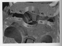
Engine Systems in Tucker, Georgia, machines hand-picked 460 blocks to accept four-bolt tongue-in-groove billet steel main caps. Main bearing webs are machined, drilled, and tapped for splayed bolts, and a tang is sized to fit into a groove in the cap. An Engine Systems stock block assembly will generate 900 horsepower—and live.
