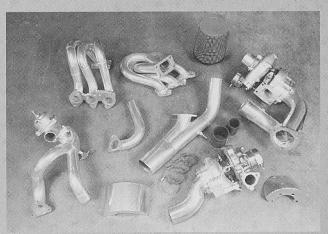
Smith's kit drives two T25/T28 Garretts simultaneously from their own three-cylinder header. Ideally, the turbos would deliver full boost at 3,500 rpm. Braided stainless-steel hoses were used to route engine oil from the original ports to the new turbos.
