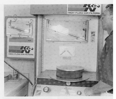
Contrary to what you may have been told or sold, air filters do not make horsepower. A paper air filter will not restrict airflow into the engine if it is properly sized. An undersized air filter can restrict airflow and power. The material that the filtering medium is made out of is of little concern as long as it filters dirt particles out of the air-charge.
