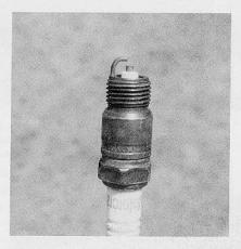
Install a spark plug with a shortened negative electrode and a .030- to .035-inch gap. A standard (long) negative electrode shrouds the spark and can become a glow plug if it absorbs enough heat. The superheated electrode can ignite the fuel early, causing detonation.
