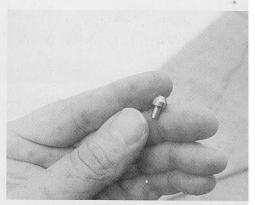
The number on the jet indicates the size of the orifice, as with carburetor jets.
