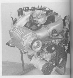
Magnuson's GM 5.3-liter Magna Charger kit is equally impressive. The self-adjusting single serpentine belt arrangement further reduces installation time. All MC kits are complete, including illustrated installation instructions. Applications include 1999–2000 Chevrolet Silverado, 2000 Chevrolet Tahoe, 2000 Chevrolet Suburban, 1999–2000 GMC Sierra, 2000 GMC Yukon, and 2000 GMC Yukon LX.
