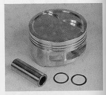
Custom pistons are a marvel of modern engineering and manufacturing techniques. This example features an oversized dish, exacting valve divots, a short wrist pin for weight savings, spiral pin locks, minimal skirt area, and a comparatively short compression height to accommodate a long connecting rod and/or a long (stroked) crank throw.
