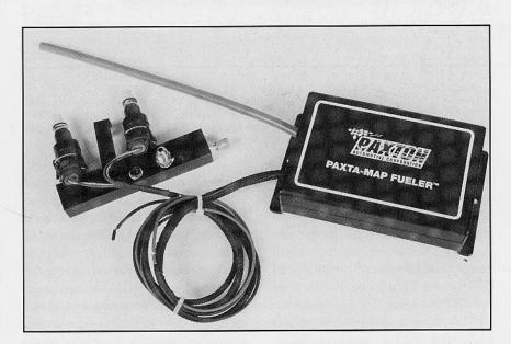
One of Paxton's supplemental fuel delivery systems is designed around a programmable microprocessor called Paxta-Map. Depending on the application, some Paxton supercharger kits include a PM, which provides a separate fuel map for up to three auxiliary injectors.
