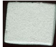
Figure 1: Macroscopic image of the sample, deposited layer – Babbitt.
