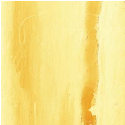
Figure 4: Topographical image of the surface for one of the fields of an eucalyptus veneer analyzed by CLSM.
