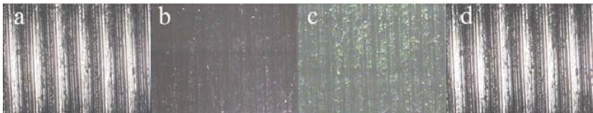
Figure 5: Machined surface image (Fig. 4b): two-sided lighting with the use of halogen – (1-3). One-sided lighting with the use of blue LED – (2), one-sided lighting with the use of green LED – (4). Four-sided lighting with the use of halogen and LED – (1-2-3-4).
