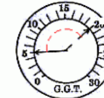
Head Gasket Leak Floats between 5-9".
