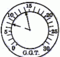
Improper Idle Mixture Floats between 8-14"
