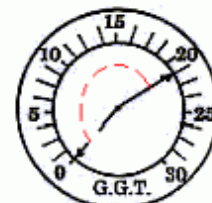
Worn Rings Diluted Oil Drops to 0", then rises to 22" when accelerator is rapidly depressed and released.
