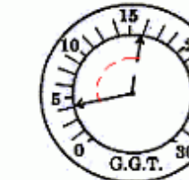
Restricted Exhaust System Normal when first started Drops to as low as 4" and stabilizes.
