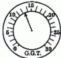
Late Ignition Timing 10-17" at idle. Normal cam.
