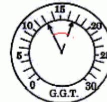
Worn Valve Guides Oscillates around 4"
