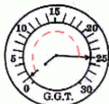
Normal Reading Drops to 2", then rises to 25" When accelerator is rapidly depressed and released.
