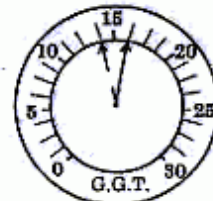
Small Spark Gap or Defective Points Slight float between 14-15".
