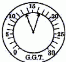
Burned or Warped Valve Regular, even spaced down-scale flick around 4"
