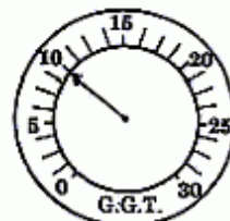
Late Valve Timing 8-15" at idle
