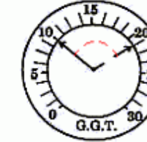
Weak Valve Springs Violent oscillation (about 10") as RPMs increase. Often steady at idle.
