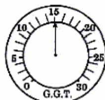
Normal Reading High lift cam w/large overlay
