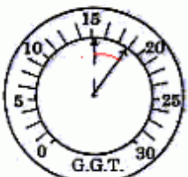
Leaky Valve Regular drop of about 2".
