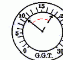
Sticking Valves Normally steady. Intermittently flicks downward around 4".
