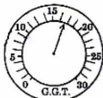
Normal Reading 14-20" at idle
