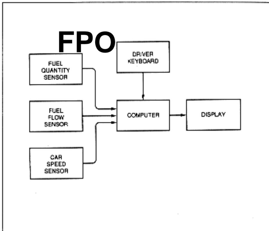
The system computes a particular trip parameter from the input data. For example, fuel economy in miles per gallon (MPG) can be found by computing
