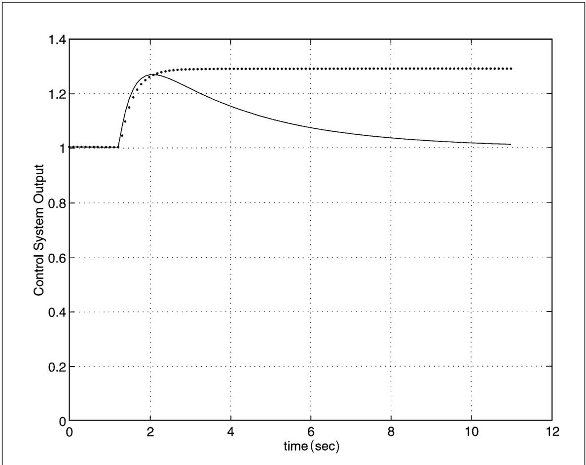
dynamic response is also affected by  $G$ . Raising the gain too far will cause the system response to become oscillatory. Often if the gain is too large, the system becomes unstable. This property of having a steady error in response to a steady disturbance is fundamental to all control systems incorporating a proportional controller, but can be eliminated by use of a proportional-integral controller.
