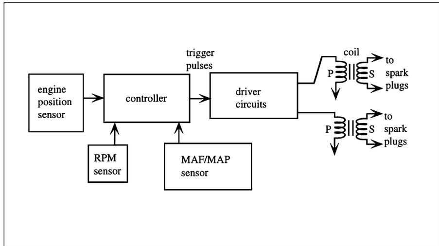
in power delivery during its power stroke. The other cylinder will be in its exhaust stroke and the spark will have no effect. Most engines have an even number of cylinders and there will be a separate driver circuit and coil for each pair of cylinders.
