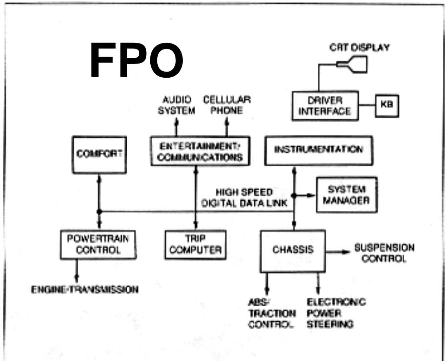
control. The driver can, for example, select to display the entertainment system operation. This display mode permits the driver to select radio, tape, or CD, and to tune the radio to the desired station and set the volume. In vehicle diagnostic mode, the CRT can be configured to display the parameters required by the mechanic for performing a diagnosis of any on-board electronic system.
