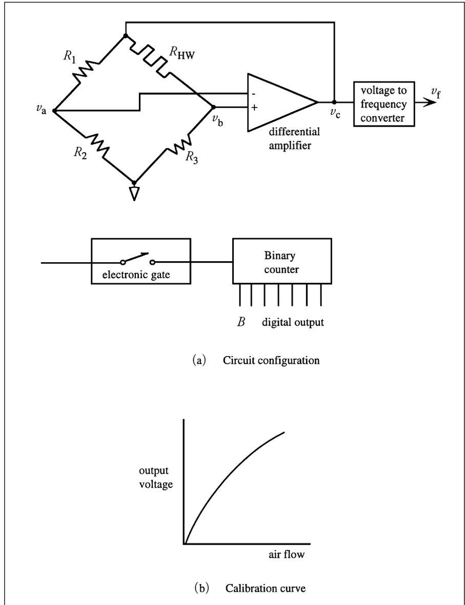
During each cycle of the electronic gate, the BC contains a binary number given by the product of the v/f frequency and the time interval. For example, if the mass air flow were such that the v/f frequency were 1000 cycles/sec and the switch were closed for .1 sec, then the BC would contain the binary equivalent of decimal 100 (i.e.,  $1000 \times .1 = 100$ ). If the mass air flow increased
