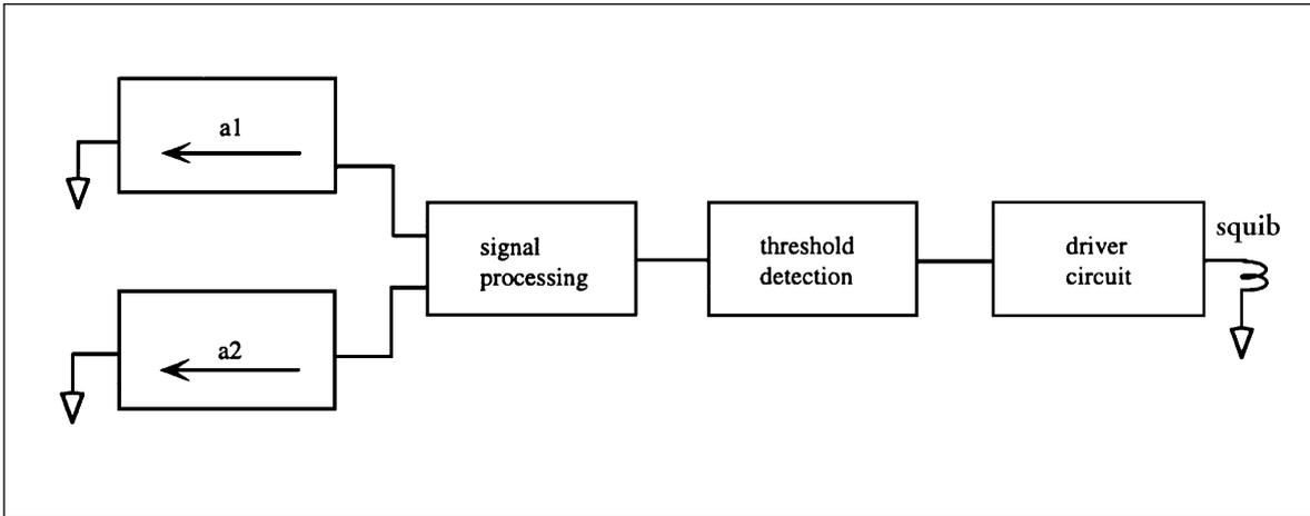
threshold, the driver circuit sends a current of sufficient strength to activate the squib and inflate the airbag.
