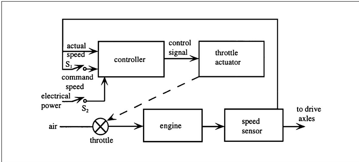
Whenever the actual speed is less than the desired speed the throttle opening is increased by the actuator, which increases vehicle speed until the error is zero, at which point the throttle opening remains fixed until either a disturbance occurs or the driver calls for a new desired speed.
