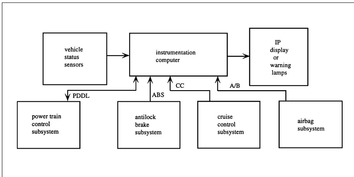
In addition to these variables, the input may include switches for detecting open doors and trunk, as well as IP selection switches for multifunction displays that permit the driver to select from various display modes or measurement units. For example, the driver may be able to select vehicle speed in miles per hour (mph) or kilometers per hour (kph).
