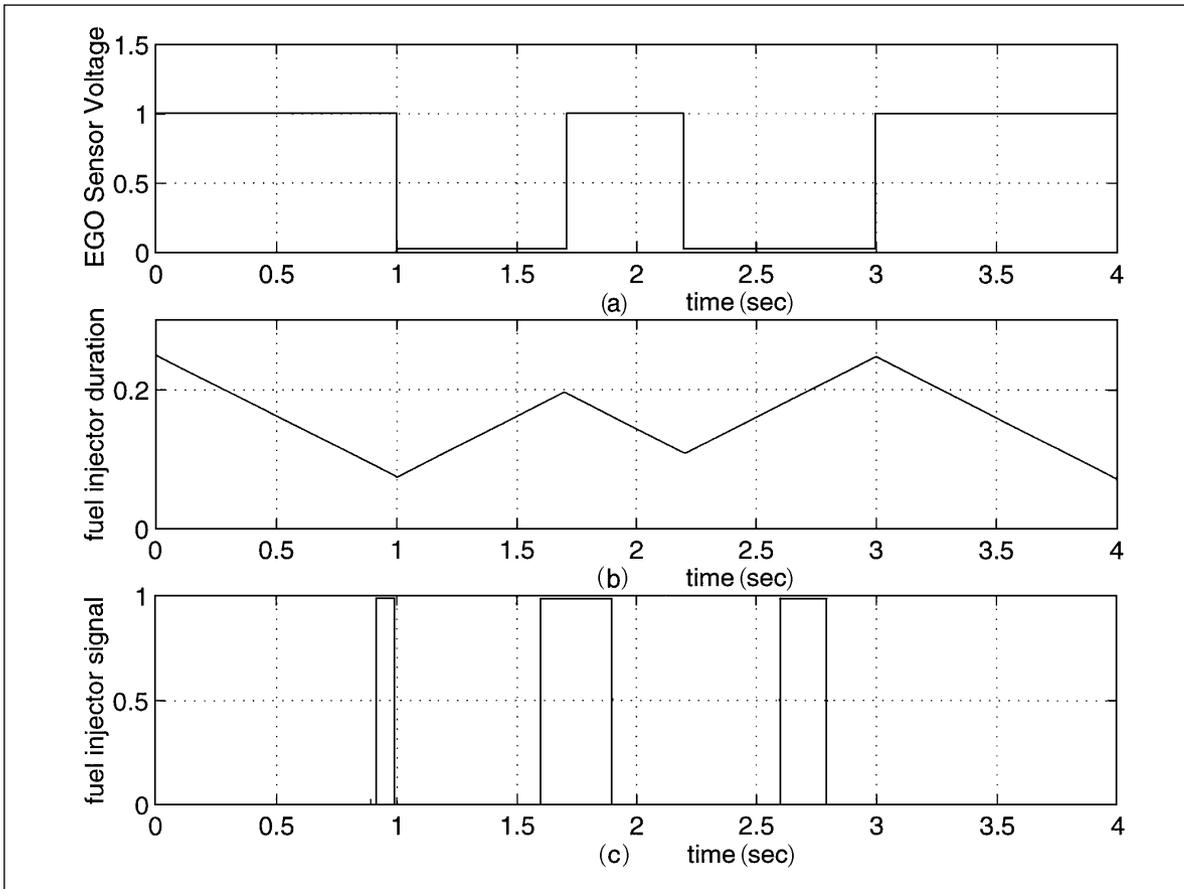
The air/fuel ratio in a closed-loop system is always increasing or decreasing in the vicinity of stoichiometry. This is in response to the EGO sensor's output, which indicates a rich or lean fuel mixture.
