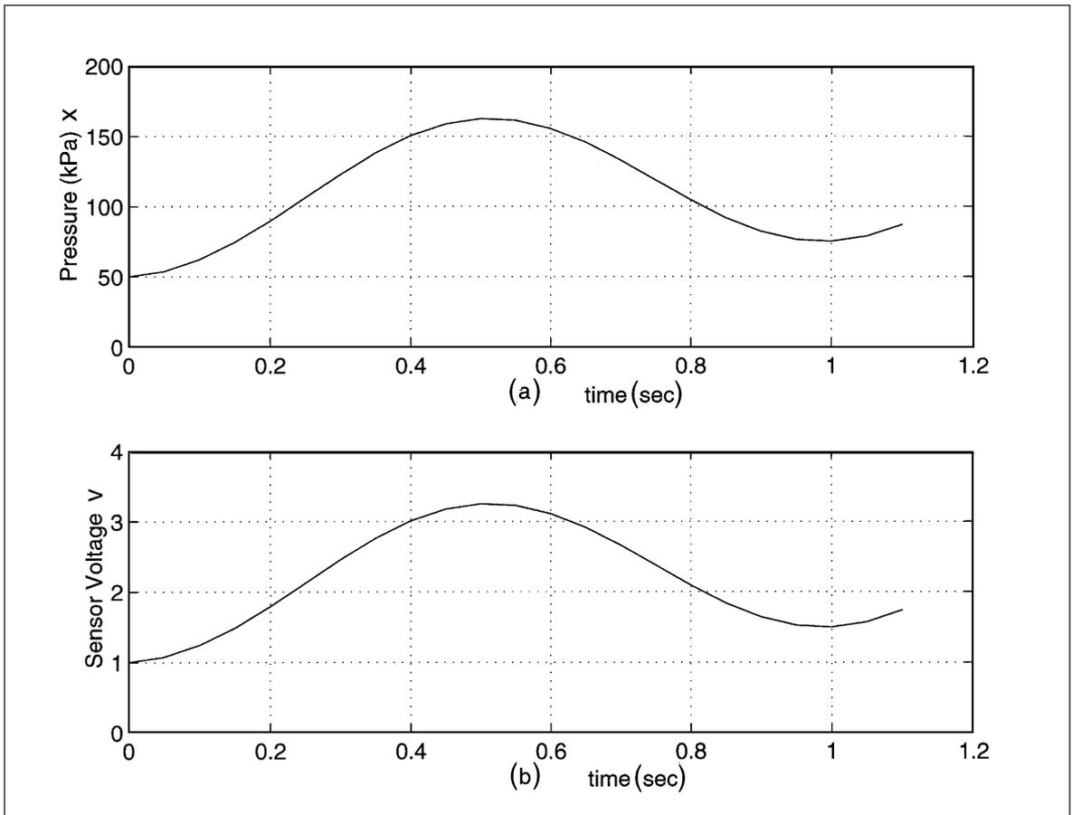
time the sensor output voltage is a multiple of the input pressure; the transducer gain is .02 volts/kPa.
