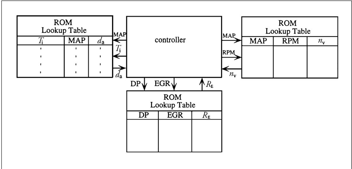
flow rate ( $R_E$ ). The volumetric efficiency is read from ROM with an address determined from RPM and MAP measurements. The intake air density is read from another section of ROM with an address determined from MAP and  $T_i$  measurements. The EGR volume flow rate is read from still another section of ROM with an address determined from differential pressure (DP) and EGR valve position. These variables are combined to yield the mass air flow rate:
