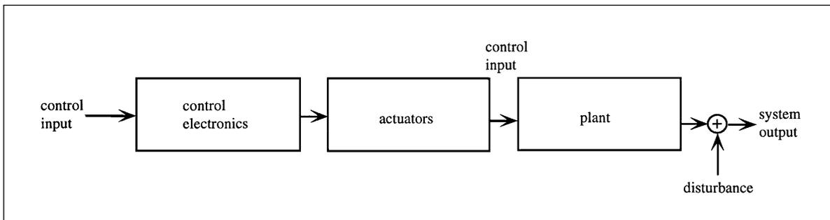
The control electronics generates the electrical signal for the actuator in response to the control input and in accordance with the desired relationship between the control input and the system output. The operation of the plant is directly regulated by the actuator (which might simply be an electric motor). The system output may also be affected by external disturbances that are not an inherent part of the plant but are the result of the operating environment.
