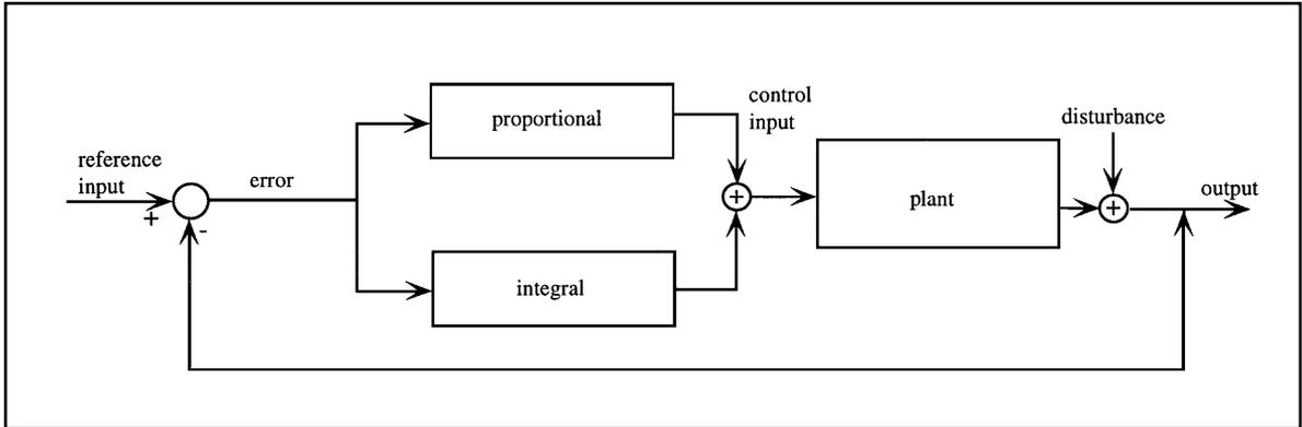
digital controllers. The relative ease and low cost of implementing PI controllers is part of the motivation for the trend toward electronic control in automotive systems.
