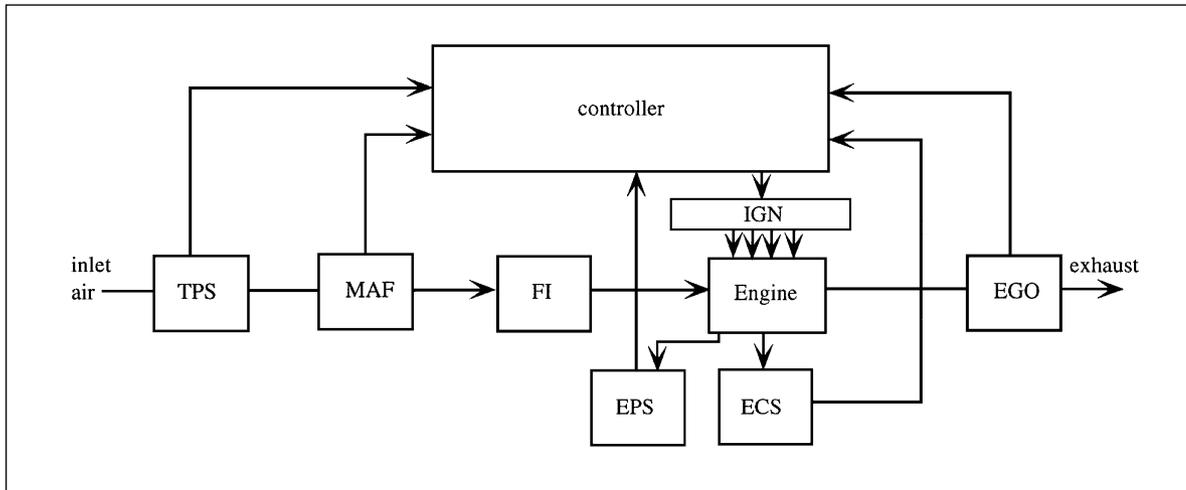
The signals from the various sensors enable the controller to determine the correct fuel flow in relation to the air flow to obtain the stoichiometric mixture. From this calculation the correct fuel delivery is regulated via fuel injectors. In addition, optimum ignition timing is determined and appropriate timing pulses are sent to the ignition control module (IGN).
