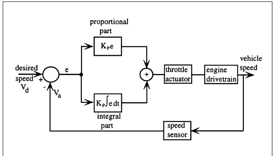
Operation of the system can be understood by first considering the operation of a proportional controller (that is, imagine that the integral term is not present for the sake of this preliminary discussion). We assume that the driver has reached the desired speed (say, 60 mph) and activated the speed set switch. If the car is traveling on a level road at the desired speed, then the error is zero and the throttle remains at a fixed position.
