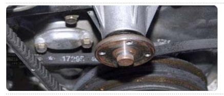
Think of the water pump as the heart of your vehicle cooling system. Its job is to continuously circulate engine coolant through the cooling system— from the radiator to the engine and then back again. If the water pump fails in this Sisyphean task the cooling system itself will fail to function. Your vehicle will run hot and possibly suffer serious damage from engine overheating.
